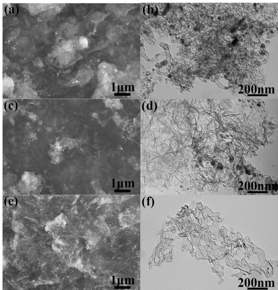
Figure S2 (a)SEM and (b) TEM images of Co, N-CNT-120; (c)SEM and (d) TEM images of Co, N-CNT-160; (e)SEM and (f) TEM images of Co, N-CNT-180.
