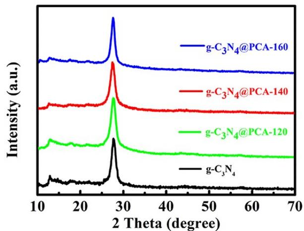
Figure S9 XRD patterns of g-C<sub>3</sub>N<sub>4</sub>@PCA-T (120 °C, 140 °C, 160 °C, 180 °C).
