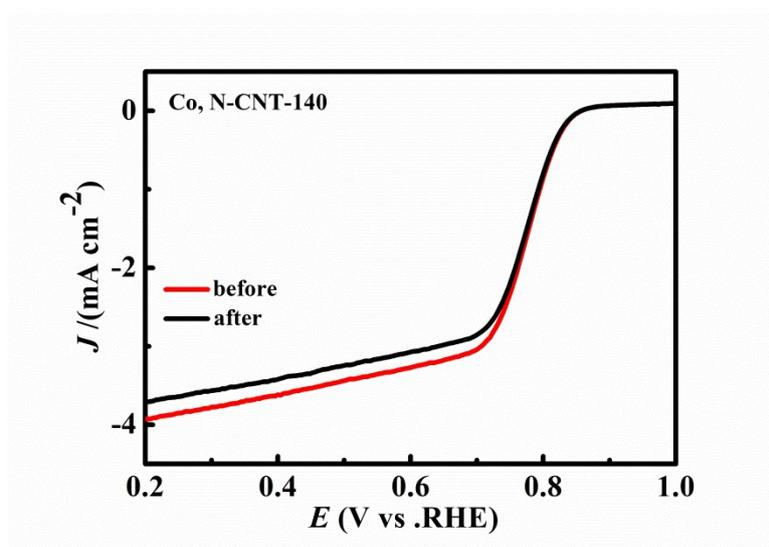
Figure S8 LSV curves of Co, N-CNT- 140 before and after 5000 cycles.
