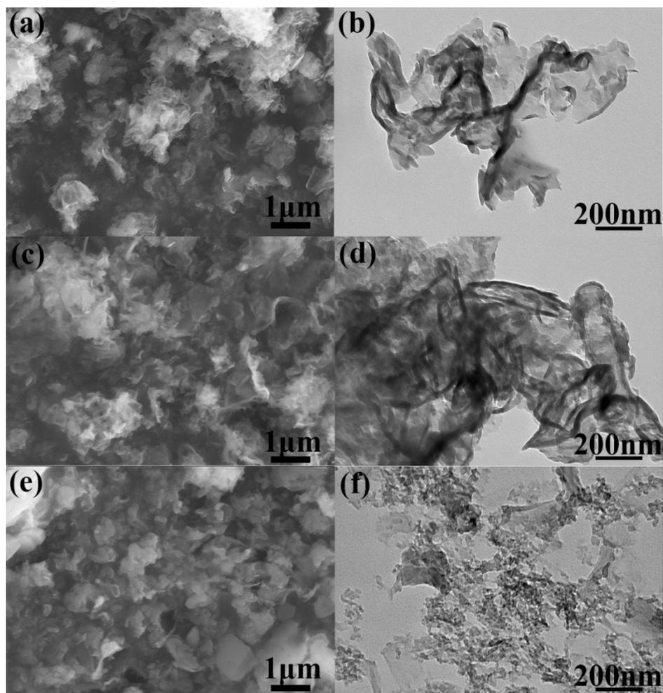
Figure S1 (a)SEM and (b)TEM images of g-C<sub>3</sub>N<sub>4</sub>/PCA-120; (c)SEM and (d)TEM images of g-C<sub>3</sub>N<sub>4</sub>/PCA-160; (e)SEM and (f)TEM images of g-C<sub>3</sub>N<sub>4</sub>/PCA-180;
