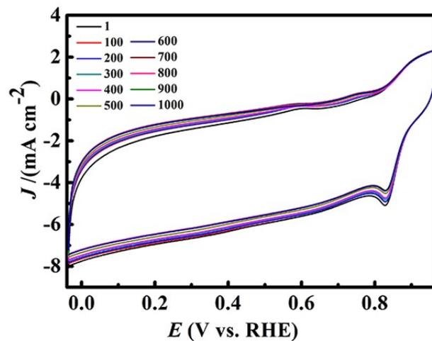
Figure S7 CV curves of Co, N-140 before and after cycling 1000 cycles in O<sub>2</sub> saturated 0.1 M KOH aqueous solution with a scan rate of 100 mV s<sup>-1</sup>.
