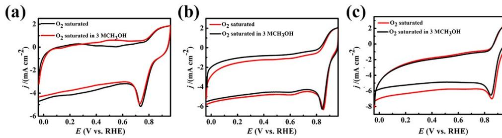
Figure S4 (a) CV of Co, N-CNT-120 in O<sub>2</sub>-saturated 0.1 M KOH solution with 3M CH<sub>3</sub>OH; (b) CV of Co, N-CNT-140 in O<sub>2</sub>-saturated 0.1 M KOH solution with 3M CH<sub>3</sub>OH; (c) CV of Co, N-CNT-160 in O<sub>2</sub>-saturated 0.1 M KOH solution with 3M CH<sub>3</sub>OH.
