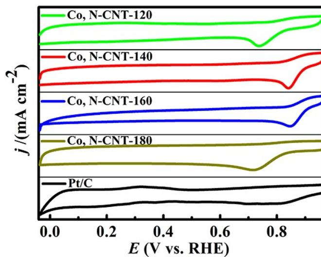
Figure S5 CV curves of Co, N-CNT-T (120 °C, 140 °C, 160 °C 180°C) and Pt/C in O<sub>2</sub> saturated 0.1 M
