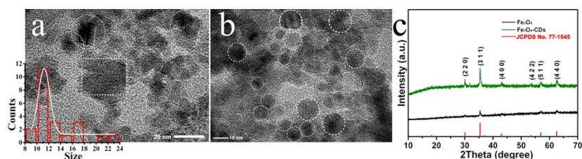
**Fig. S5** (a) TEM of  $\text{Fe}_3\text{O}_4$ , (b) HRTEM of the  $\text{Fe}_3\text{O}_4$ -CDs image in scale of 10 nm, (c) XRD analysis of the  $\text{Fe}_3\text{O}_4$ -CDs.
