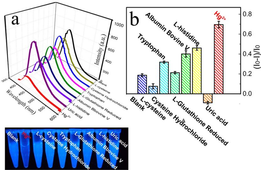
**Fig. S6.** (a) Fluorescence spectra and (b) bar diagram of different amino acids sensing. Insert: the corresponding image under UV lamp.
