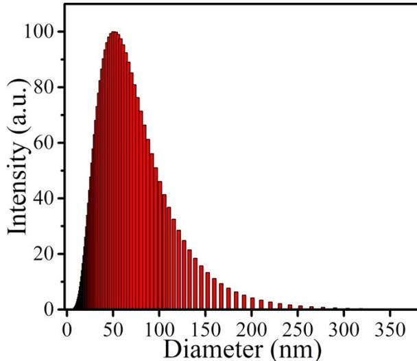
**Fig. S4** DLS analysis of the  $\text{Fe}_3\text{O}_4$ -CDs
