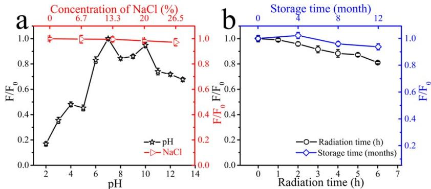
**Fig. S3** (a) Fluorescence spectra stability under different salinity and pH (b) The fluorescence quenching ratio after UV radiation exposure and storage time.
