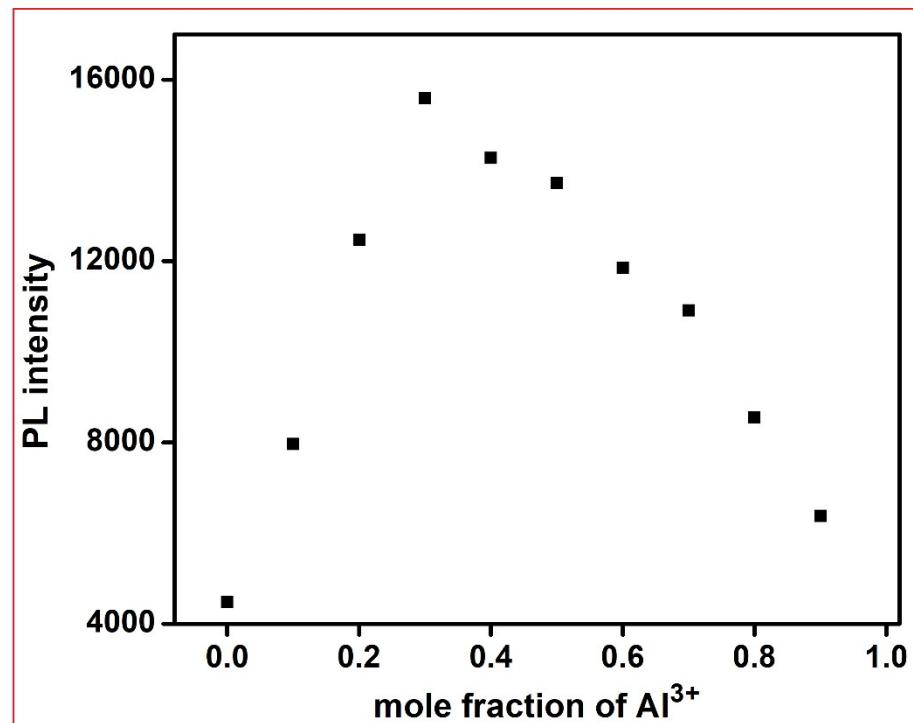
**Fig. S15.** Job's plot from emission spectra.
