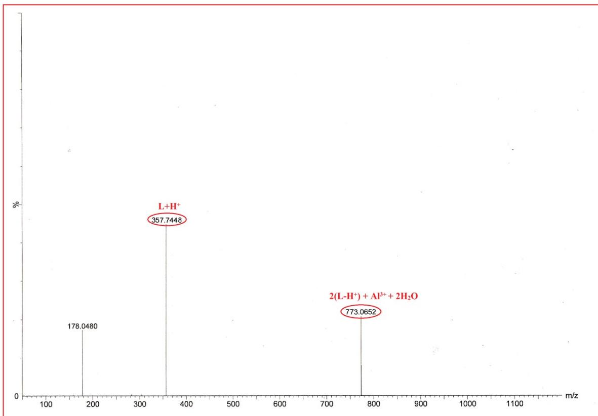
**Fig. S11.** Mass spectra of L-Al<sup>3+</sup>adduct.
