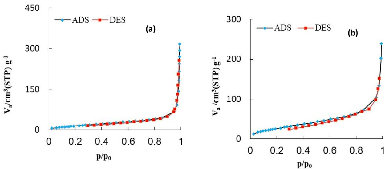
Fig. S6. Adsorption-desorption isotherm graphs for (a) PAN-PA6 (b) PAN-PA6/PANI electrospun nanofiber mats.
