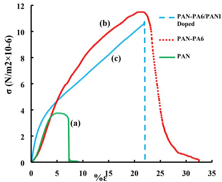
Fig. S5. The stress-strain curve of the (a) PAN; (b) PAN-PA6 and (c) PAN-PA6/PANI Doped membrane.
