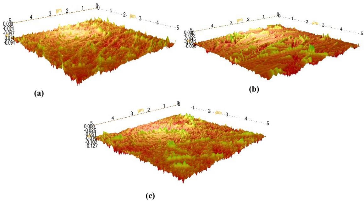
Fig. S4. AFM images of PAN-PA6/PANI electrospun nanofiber mats with (a) 45; (b) 60 and (c) 75 minutes polymerization time.
