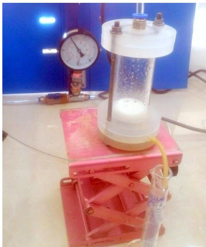
**Fig. S2. Home made set up for oil/water separation studies**
