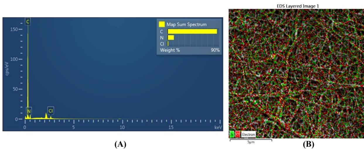
**Fig. S3. (A) FESEM-EDX spectra , (B) Mapping pattern of PAN-PA6/PANI Doped nanofibers**
