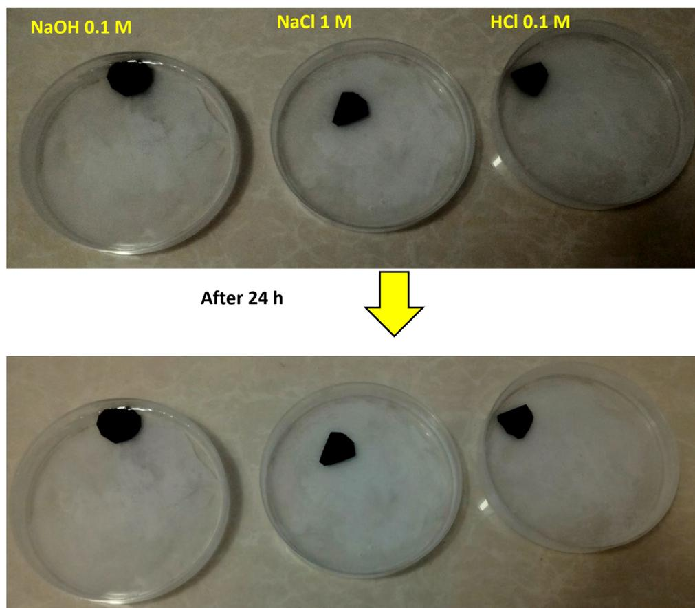
Fig. S7. Photographs of PAN-PA6/PANI Doped membranes before and after immersing in 0.1 M HCl, 1 M NaCl and 0.1 M NaOH solution for 24 h
