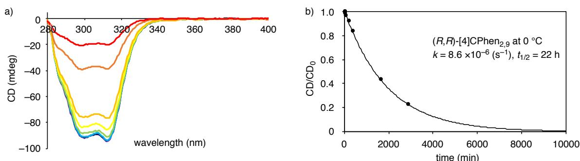
**Fig. S20.** Racemization of  $(Z,R,Z,R)$ -[4]CPhen<sub>2,9</sub> in toluene at 0 °C. (a) VT CD spectra. (b) Decay of the CD signal at 298 nm. The coefficient of ( $R^2$ ) was 0.99998 and confirmed the sufficient of fit for analysis.
