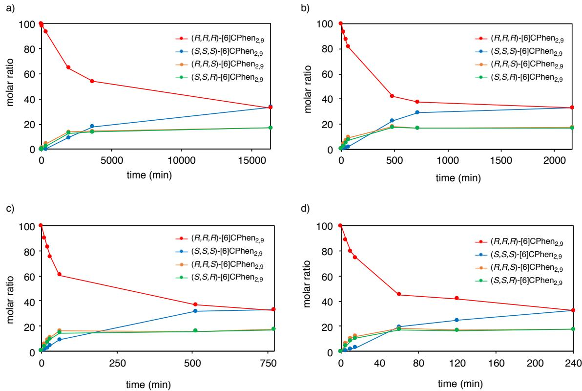
**Fig. S16.** Time-course analysis of isomerization of  $(Z,R,Z,R,Z,R)-[6]CPhen_{2,9}$  in 1,2,4-trichlorobenzene at (a) 149 °C, (b) 181 °C, (c) 191 °C, and (d) 201 °C.
