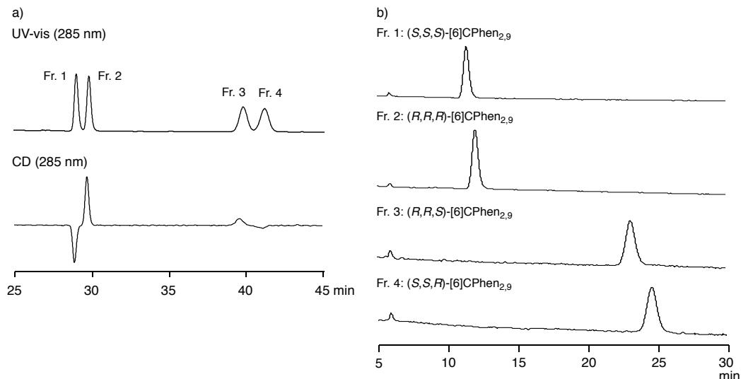
**Fig. S9.** Separation of stereoisomers of [6]CPhen<sub>2,9</sub>. (a) HPLC analysis with DAICEL CHIRALPAK IA (4.6φ × 250 mm). Conditions: eluent 50% MeOH in CHCl<sub>3</sub>, flow rate = 1.0 mL/min, column temperature = 40 °C. (b) HPLC analysis of the isolated stereoisomers.
