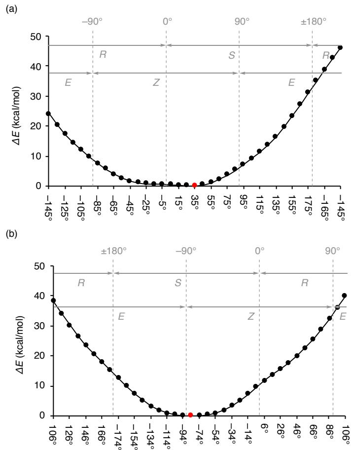
**Fig. S12.** Energy profile of 2,2'-biaryl linkage (1-2-2'-1') in (a) (*E/Z,S,Z,S,Z,R*)-[6]CPhen<sub>2,9</sub>, and (b) (*Z,S,E/Z,S,Z,R*)-[6]CPhen<sub>2,9</sub> from scan calculations at the semiempirical PM6 level of theory. Red dots show stationary points.
