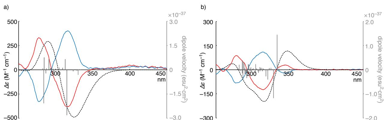
**Fig. S11.** CD spectra of (a) (*Z,S,Z,S,Z,S*)/(*Z,R,Z,R,Z,R*)-[6]CPhen<sub>2,9</sub>, and (b) (*Z,S,Z,S,Z,R*)/(*Z,R,Z,R,Z,S*)-[6]CPhen<sub>2,9</sub>. The dotted line and gray bars show the simulated CD spectrum and the rotatory velocity of (a) (*Z,R,Z,R,Z,R*)-[6]CPhen<sub>2,9</sub> and (b) (*Z,R,Z,R,Z,S*)-[6]CPhen<sub>2,9</sub>, respectively, as calculated by TD DFT at the B3LYP/6-31G(d,p) level of theory.
