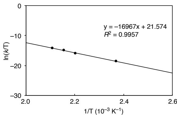
**Fig. S18.** Eyring plot for the isomerization of  $(Z,R,Z,R,Z,R)$ -[6]CPhen<sub>2,9</sub> to reveal the activation energy with  $\Delta H^\ddagger = +33.7$  kcal/mol,  $\Delta S^\ddagger = -4.4$  kcal/mol·K, and  $\Delta G^\ddagger = +35.0$  kcal/mol at 25 °C.
