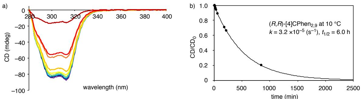
**Fig. S21.** Racemization of  $(Z,R,Z,R)$ -[4]CPhen<sub>2,9</sub> in toluene at 10 °C. (a) VT CD spectra. (b) Decay of the CD signal at 298 nm. The coefficient of ( $R^2$ ) was 0.99994 and confirmed the sufficient of fit for analysis.
