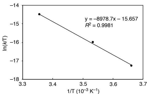
**Fig. S23.** Eyring plot for racemization of  $(Z,R,Z,R)$ -[4]CPhen<sub>2,9</sub> to reveal the activation energy with  $\Delta H^\ddagger = +17.8 \text{ kcal/mol}$ ,  $\Delta S^\ddagger = -16.2 \text{ kcal/mol}\cdot\text{K}$ , and  $\Delta G^\ddagger = +22.7 \text{ kcal/mol}$  at 25 °C.
