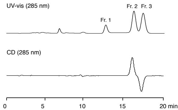
**Fig. S7.** HPLC analysis of [4]CPhen<sub>2,9</sub> with COSMOSIL Cholester (4.6φ × 250 mm). Conditions: eluent 50% MeOH in CHCl<sub>3</sub>, flow rate = 1.0 mL/min, column temperature = 25 °C.
