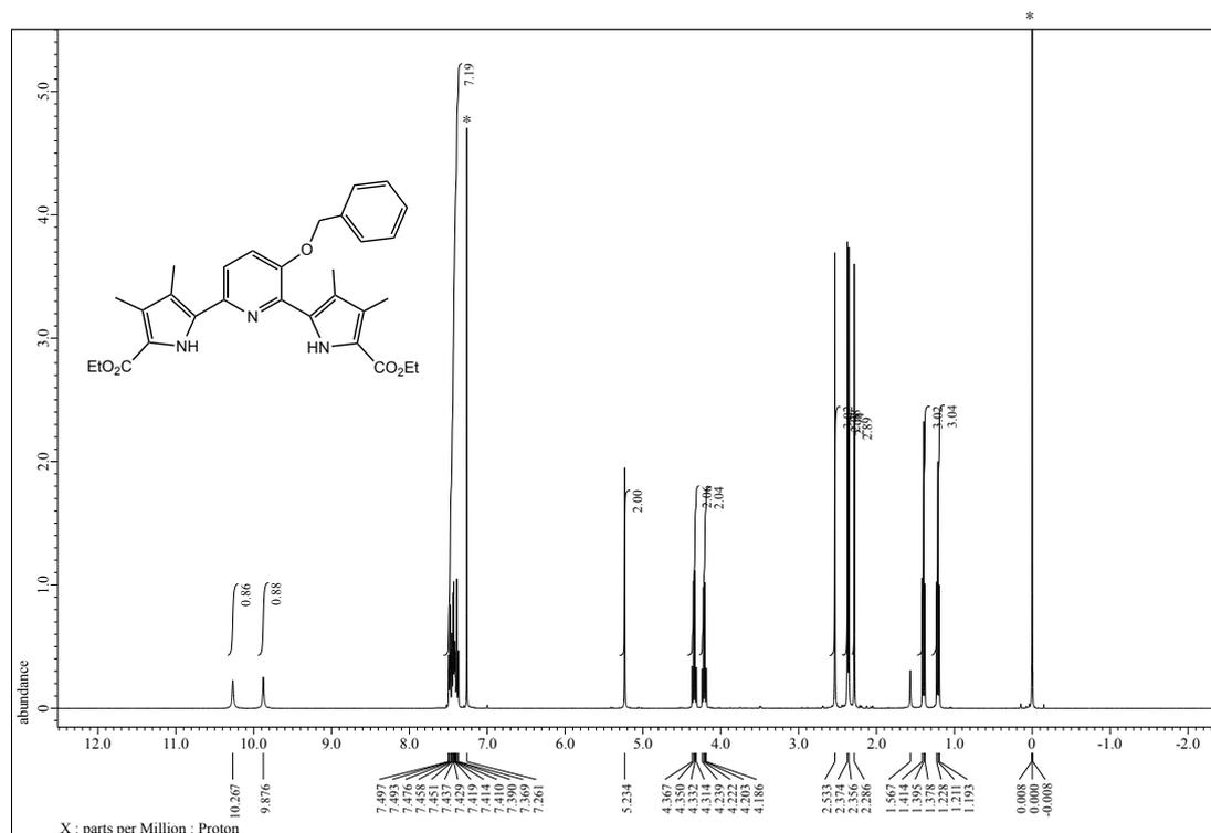
**Fig. S5.** <sup>1</sup>H NMR spectrum of **6** in CDCl<sub>3</sub> at 25 °C. \* indicates CHCl<sub>3</sub> and TMS.
