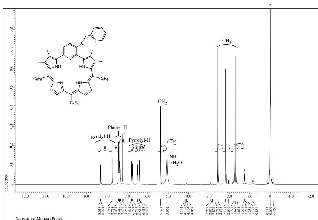
**Fig. S11.**  $^1\text{H}$  NMR spectrum of **1** in  $\text{CDCl}_3$  at  $25\text{ }^\circ\text{C}$ . \* indicates residual solvents and TMS.
