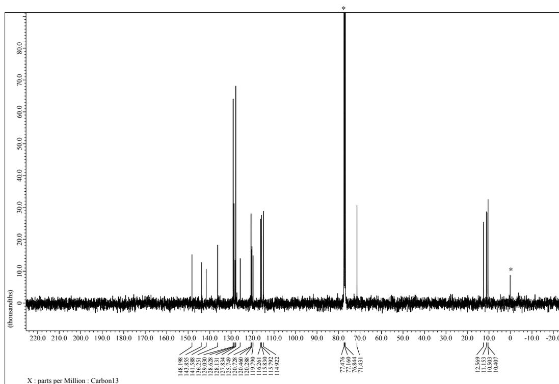
**Fig. S10.** <sup>13</sup>C NMR spectrum of **8** in CDCl<sub>3</sub> at 25 °C. \* indicates CDCl<sub>3</sub> and TMS.
