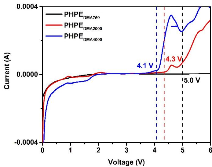
**Figure S8.** Linear sweep voltammetry (LSV) of  $\text{PHPE}_{\text{DMA}750}$ ,  $\text{PHPE}_{\text{DMA}2000}$ , and  $\text{PHPE}_{\text{DMA}4000}$  at 60 °C.
