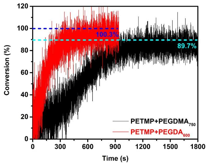
**Figure S7.** Kinetics of the initiator-free thiol-ene photopolymerization with different unsaturated bonds.
