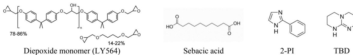
Sebacic acid and TBD were added to the epoxy as received, and mixed for 24 h at 50°C until obtaining a white homogeneous mixture. The final mixture was then placed into an open mould, degassed under vacuum for 2h at 90°C to ensure removal of air inadvertently added during mixing. Samples were then cured at 145°C for 8h (ramp 1.7°C/min from room temperature to 145°C), a post-cure was then completed at 160°C for 8h.
