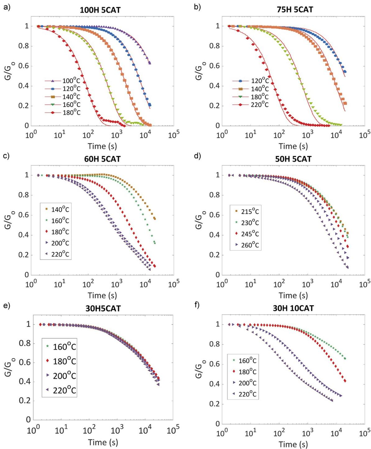
Fig. S7 Stress relaxation results obtained by DMA in shear geometry: a) 100H 5CAT, b) 75H 5 CAT c) 60H5CAT, d) 50H5CAT, e) 30H5CAT, and d) 30H10CAT
