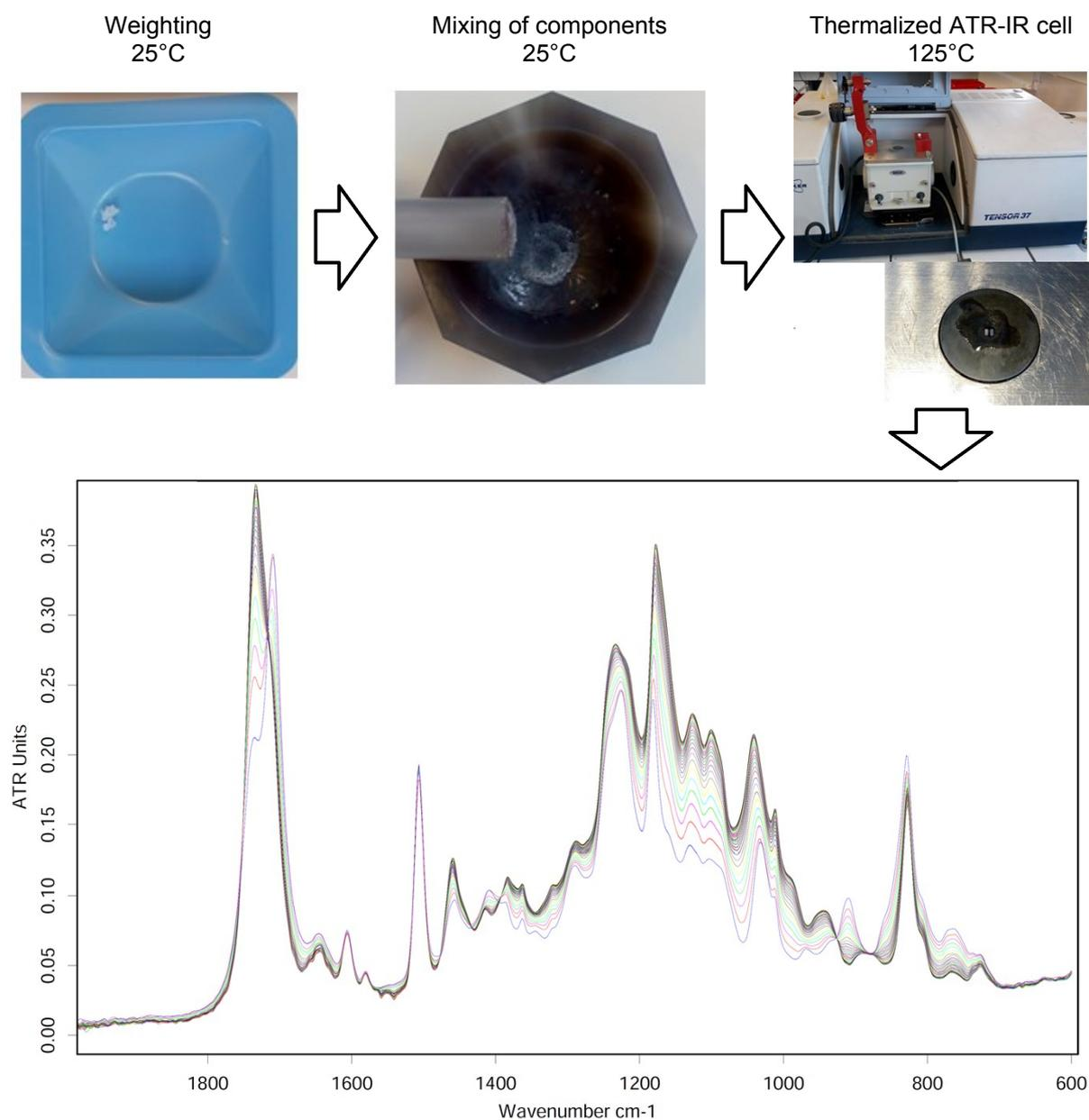
Fig. S2 Schematic of ATR-IR curing experiment to record species evolution over time.
