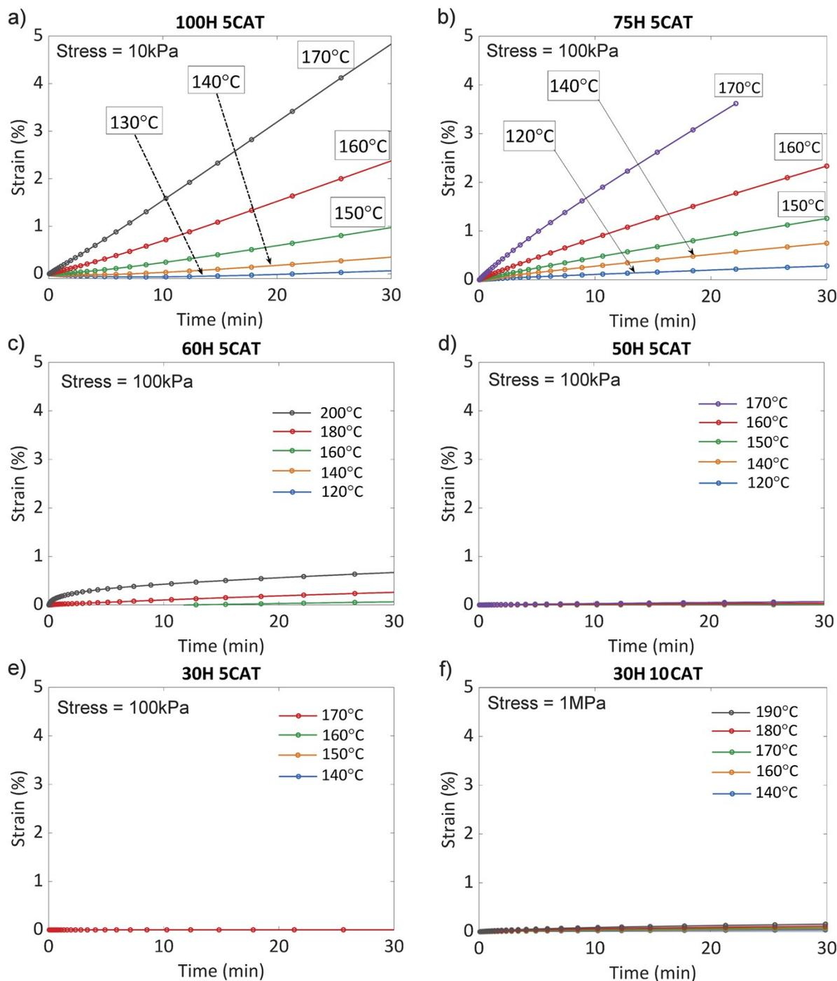
Fig. S8 Creep results for all samples
