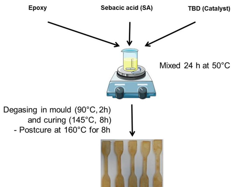
Fig. S1 Schematic of fabrication method used to produce vitrimer samples
