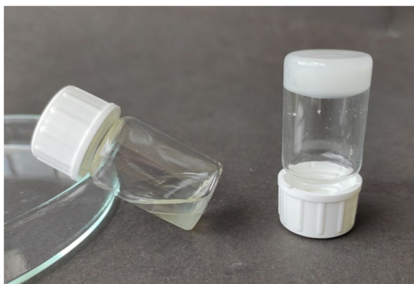
Fig. S5 Vial inversion of PZLL 80-5.5* (left) and PBLG 80-3* (right), both without the L-cystine crosslinker, after 72 h of polymerization.
