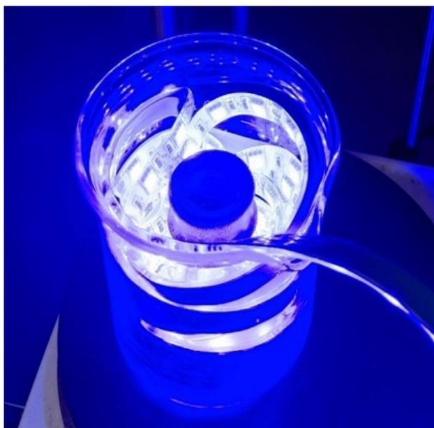
**Figure S22.** Photograph of the apparatus used for RAFT removal using a 50 LED strip (452 nm). Intensity was measured as 0.3 mW/cm<sup>2</sup> from 5 clustered LEDs at a distance of 0.5 cm.
