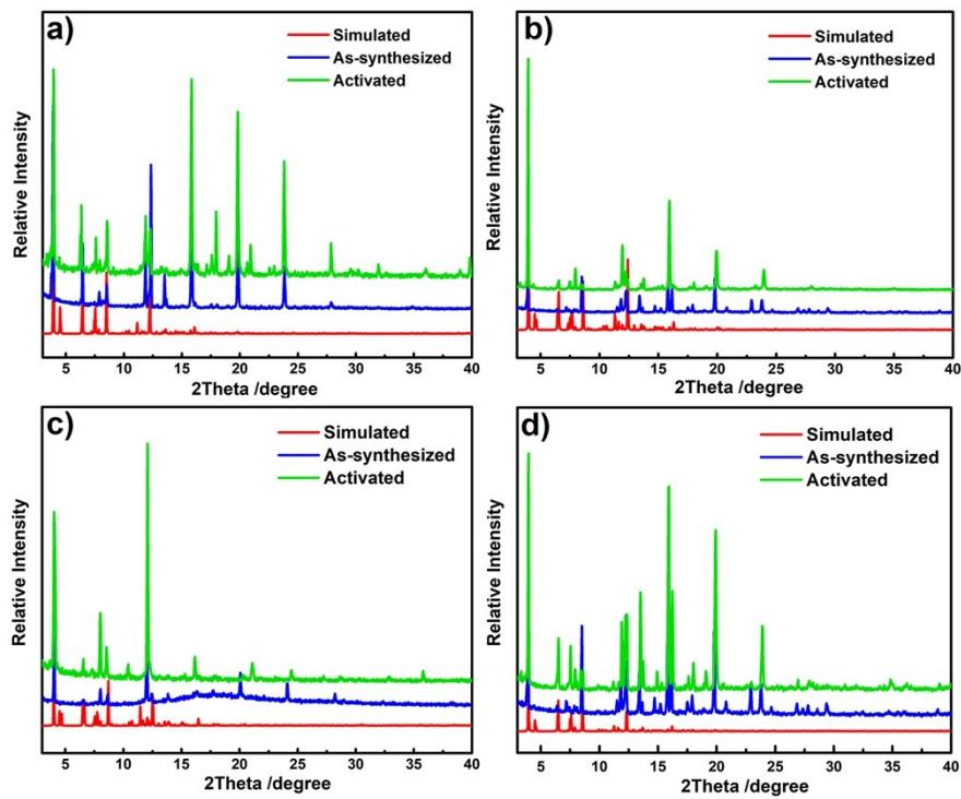
**Figure S3.** PXRD patterns for (a) JLU-Liu20, (b) JLU-Liu21, (c) JLU-Liu22 and (d) JLU-Liu46.
