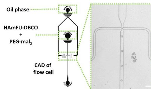
Figure S4: Microfluidic water-in-oil (W/O) emulsion preparation containing HAmFU-DBCO-DNA, pre-functionalized with NTA-mal, and PEG-mal<sub>2</sub> as crosslinker. Microfluidic device design (left) for producing tailor-made emulsion droplets. Scale bar indicates 50  $\mu\text{m}$ .
