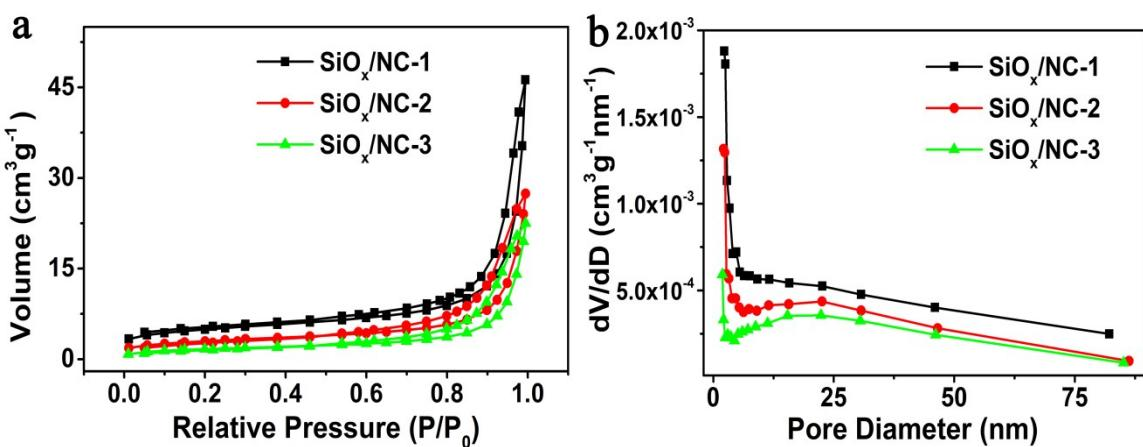
Fig. S6.  $\text{N}_2$  adsorption-desorption isotherms (a) and pore size distribution (b) of  $\text{SiO}_x/\text{NC}$  microspheres.
