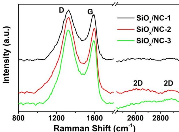
Fig. S5. Raman spectra of  $\text{SiO}_x/\text{NC-1}$ ,  $\text{SiO}_x/\text{NC-2}$  and  $\text{SiO}_x/\text{NC-3}$ .
