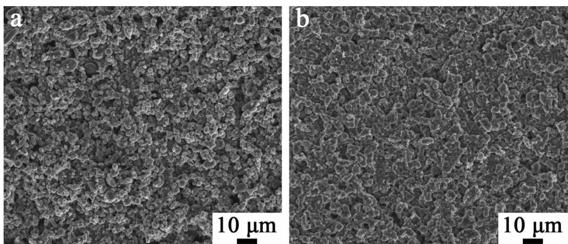
Fig. S11. SEM images of  $\text{SiO}_x/\text{NC}$ -2 electrode before (a) and after 100 cycles (b).
