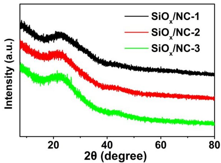
Fig. S4. XRD patterns of  $\text{SiO}_x$ /NC-1,  $\text{SiO}_x$ /NC-2 and  $\text{SiO}_x$ /NC-3.
