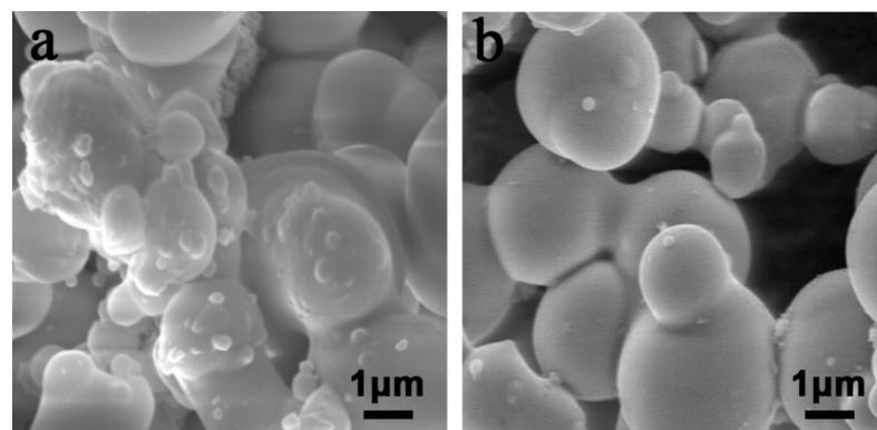
Fig. S3. SEM image of  $\text{SiO}_x$ /organosilica-3(a) and  $\text{SiO}_x$ /NC-3(b).
