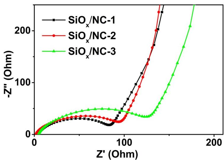
Fig. S9. EIS spectra of  $\text{SiO}_x/\text{NC}$  half cells.
