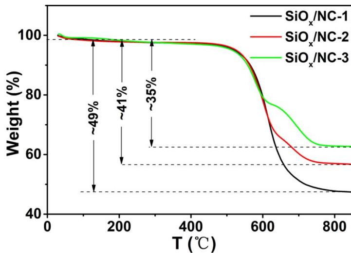
Fig. S7. TGA curves of  $\text{SiO}_x/\text{NC}$  microspheres.
