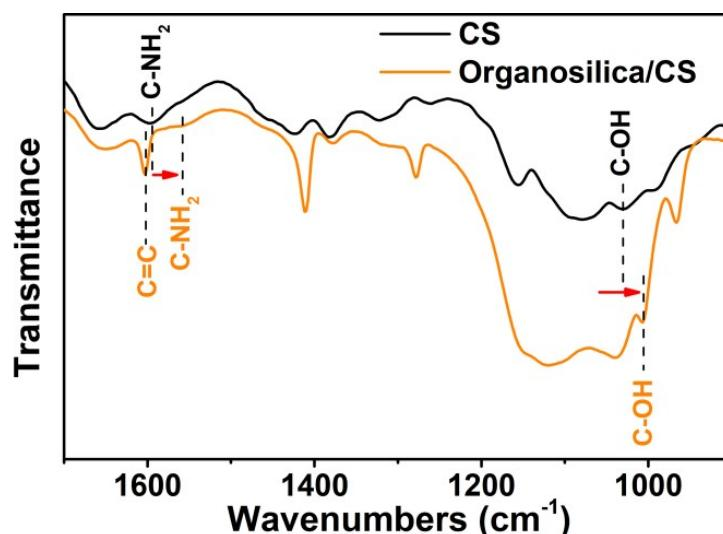
Fig. S1. FTIR spectra of raw CS and organosilica/CS composite.
