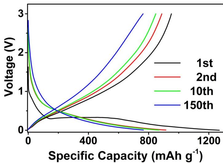
Fig. S10. Charge-discharge curves of  $\text{SiO}_x/\text{NC-2}$  at  $0.1 \text{ A g}^{-1}$ .
