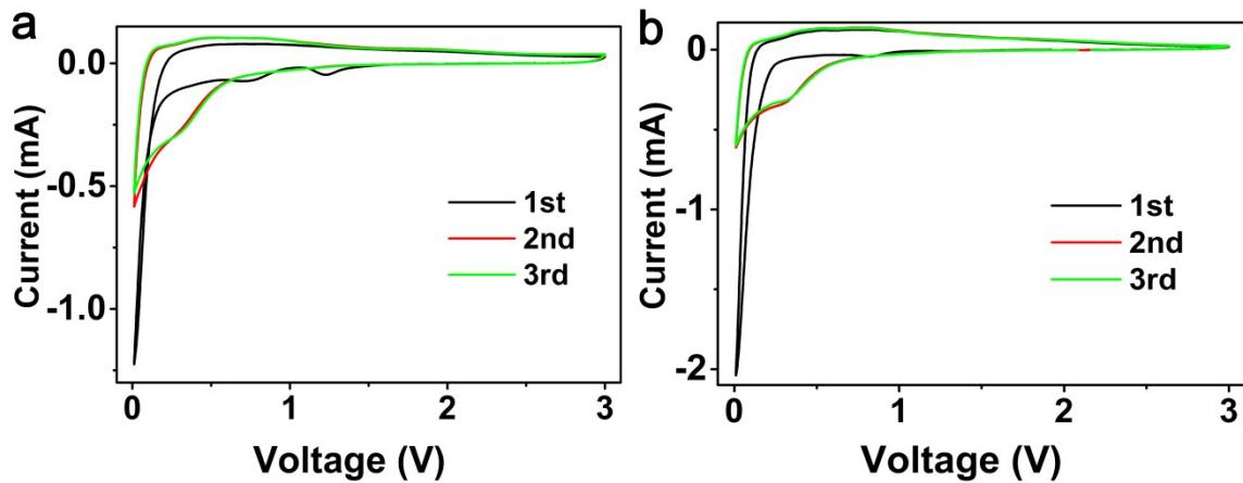
Fig. S8. CV curves of  $\text{SiO}_x/\text{NC-1}$  (a) and  $\text{SiO}_x/\text{NC-3}$  (b).
