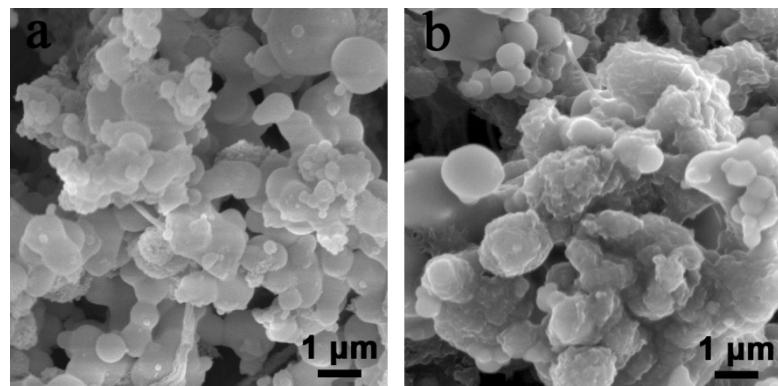
Fig. S2. SEM image of  $\text{SiO}_x$ /organosilica-1(a) and  $\text{SiO}_x$ /NC-1(b).
