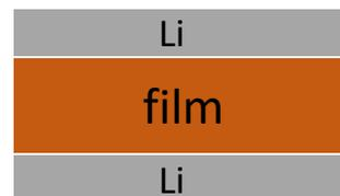
**Figure D1.** Scheme of the cell for the  $t_+$  measurement
