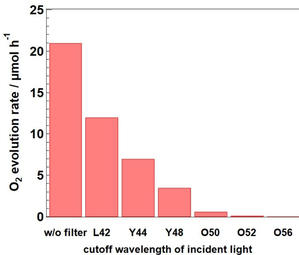
Figure S6 Dependence of the initial oxygen evolution rate of In-Fe(15%) oxide on the cutoff wavelength of the incident light. Catalyst: 100 mg, 20 mM AgNO<sub>3</sub>: 300 mL, light source: 300 W Xe arc lamp attached with cut off filters.
