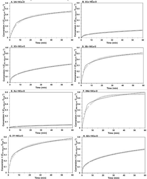
**Figure S4.** Raw data of the first carbonation (hollow circles) of A. 3Al-10Ca-O, B. 3Co-10Ca-O, C. 3Cr-10Ca-O, D. 3Er-10Ca-O, E. 3Li-10Ca-O, F. 3Nd-10Ca-O, G. 3Y-10Ca-O, H. 3Zn-10Ca-O sorbents with the optimized RPM fit used to determine  $k_{RPM}$  and  $D_{RPM}$  parameters. The experiment was carried out at in 200 sccm of 10% CO<sub>2</sub> at 873 K for 1 hr.
