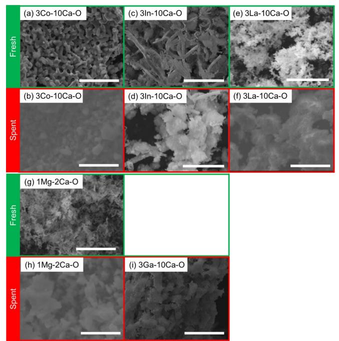
**Figure S1.** SEM images of (a) 3Co-10Ca-O fresh, (b) 3Co-10Ca-O post 11 cycles, (c) 3In-10Ca-O fresh,(d) 3In-10Ca-O post 16 cycles, (e) 3La-10Ca-O fresh, (f) 3La-10Ca-O post 11 cycles,(g) 1Mg-2Ca-O fresh,(h) 1Mg-2Ca-O post 16 cycles, (i) 3Ga-10Ca-O post 16 cycles. Samples bordered with green are fresh, samples bordered in red are post cycle samples, the white scale bar represents  $5\mu m$ .
