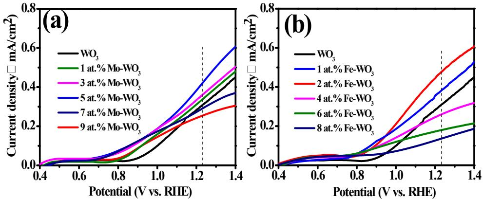
Fig. S2 LSV plots of WO<sub>3</sub> photoanodes with different Mo doping amounts (a) and with different Fe doping amounts (b) measured in 0.2 M Na<sub>2</sub>SO<sub>4</sub> solution under AM 1.5 G illumination
