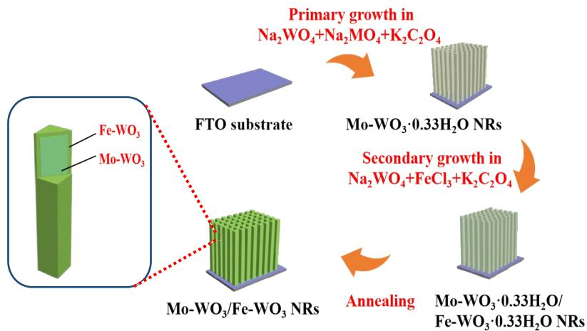
Fig. S1 Schematic illustration for the fabrication process of Mo-WO<sub>3</sub>/Fe-WO<sub>3</sub> homojunction photoanode
