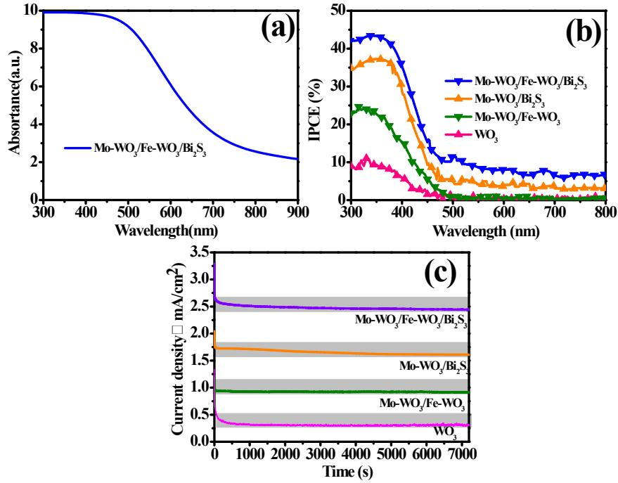
Fig. S9 (a) UV-Vis absorption spectrum of Mo-WO<sub>3</sub>/Fe-WO<sub>3</sub>/Bi<sub>2</sub>S<sub>3</sub>. (b) IPCEs plots. (c) Time-dependent photocurrent density curves of WO<sub>3</sub>, Mo-WO<sub>3</sub>/Fe-WO<sub>3</sub>, Mo-WO<sub>3</sub>/Bi<sub>2</sub>S<sub>3</sub> and Mo-WO<sub>3</sub>/Fe-WO<sub>3</sub>/Bi<sub>2</sub>S<sub>3</sub> photoanodes measured at 1.23V vs. RHE under simulated sunlight illumination for 7200 s
