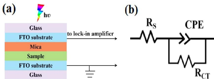
Fig. S6 (a) Schematic diagram of SPV measurement configuration. (b) The equivalent circuit of electrochemical impedance spectroscopy
