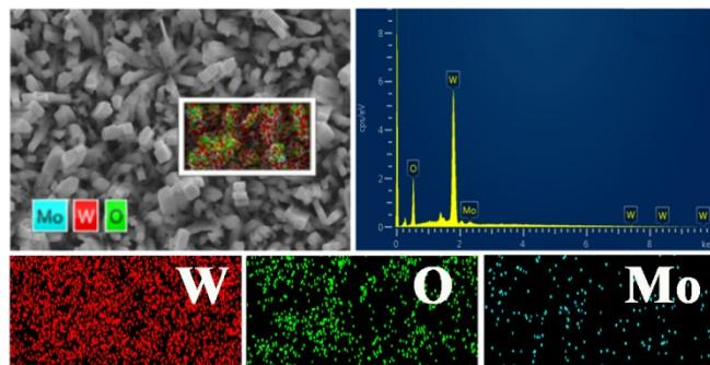
Fig.S4 EDS elemental analysis spectrum and corresponding elemental mapping images of W, O and Mo in  $\text{Mo-WO}_3$ , respectively
