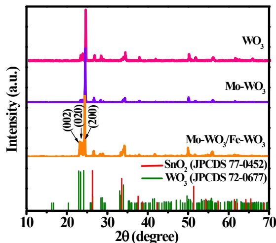
Fig. S3 XRD patterns of WO<sub>3</sub>, Mo-WO<sub>3</sub> and Mo-WO<sub>3</sub>/Fe-WO<sub>3</sub> homojunction
