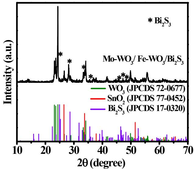
Fig. S7 XRD pattern of Mo-WO<sub>3</sub>/Fe-WO<sub>3</sub>/Bi<sub>2</sub>S<sub>3</sub>. Bottom peaks are standard positions of SnO<sub>2</sub>, WO<sub>3</sub> and Bi<sub>2</sub>S<sub>3</sub>
