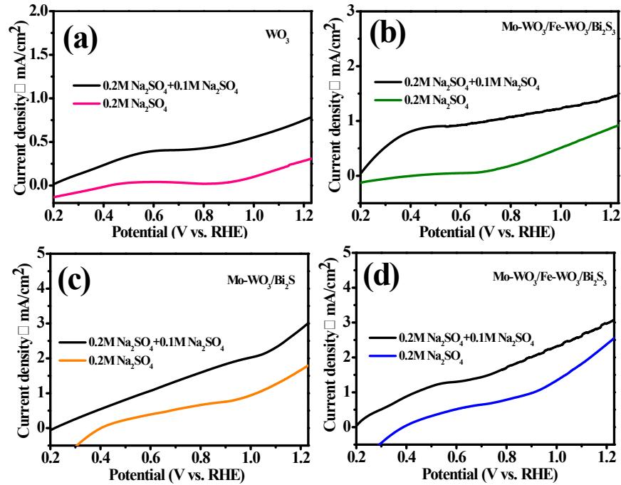
Fig. S10 LSV curves of WO<sub>3</sub>, Mo-WO<sub>3</sub>/Fe-WO<sub>3</sub>, Mo-WO<sub>3</sub>/Bi<sub>2</sub>S<sub>3</sub> and Mo-WO<sub>3</sub>/Fe-WO<sub>3</sub>/Bi<sub>2</sub>S<sub>3</sub> photoanodes measured in 0.2 M Na<sub>2</sub>SO<sub>4</sub> electrolyte solution with the addition of 0.1 M Na<sub>2</sub>SO<sub>3</sub>
