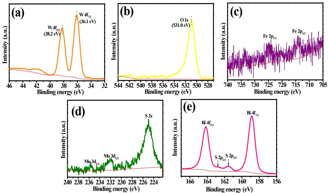
Fig. S8 High resolution XPS spectra of (a) W 4f, (b) O 1s, (c) Fe 2p, (d) Mo 3d and S 2s and (e) Bi 4f and S 2p for Mo-WO<sub>3</sub>/Fe-WO<sub>3</sub>/Bi<sub>2</sub>S<sub>3</sub> composite
