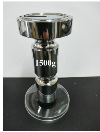
Fig. S6. Camera photographs of SPCF under the weight of 1500 g ( $\sim 2.07 \times 10^4$  Pa).
