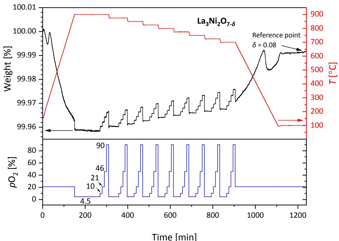
**Figure S12** — Weight loss curve for  $\text{La}_3\text{Ni}_2\text{O}_{7-\delta}$  on cooling from 900 °C to 700 °C, with intervals of 25 °C, at different  $p\text{O}_2$  values. The reference point was selected after equilibration for 3 h at  $T = 100$  °C and  $p\text{O}_2 = 0.21$  bar. The corresponding value ( $\delta = 0.08$ ) was determined by reduction in hydrogen (16%  $\text{H}_2/\text{Ar}$ ).
