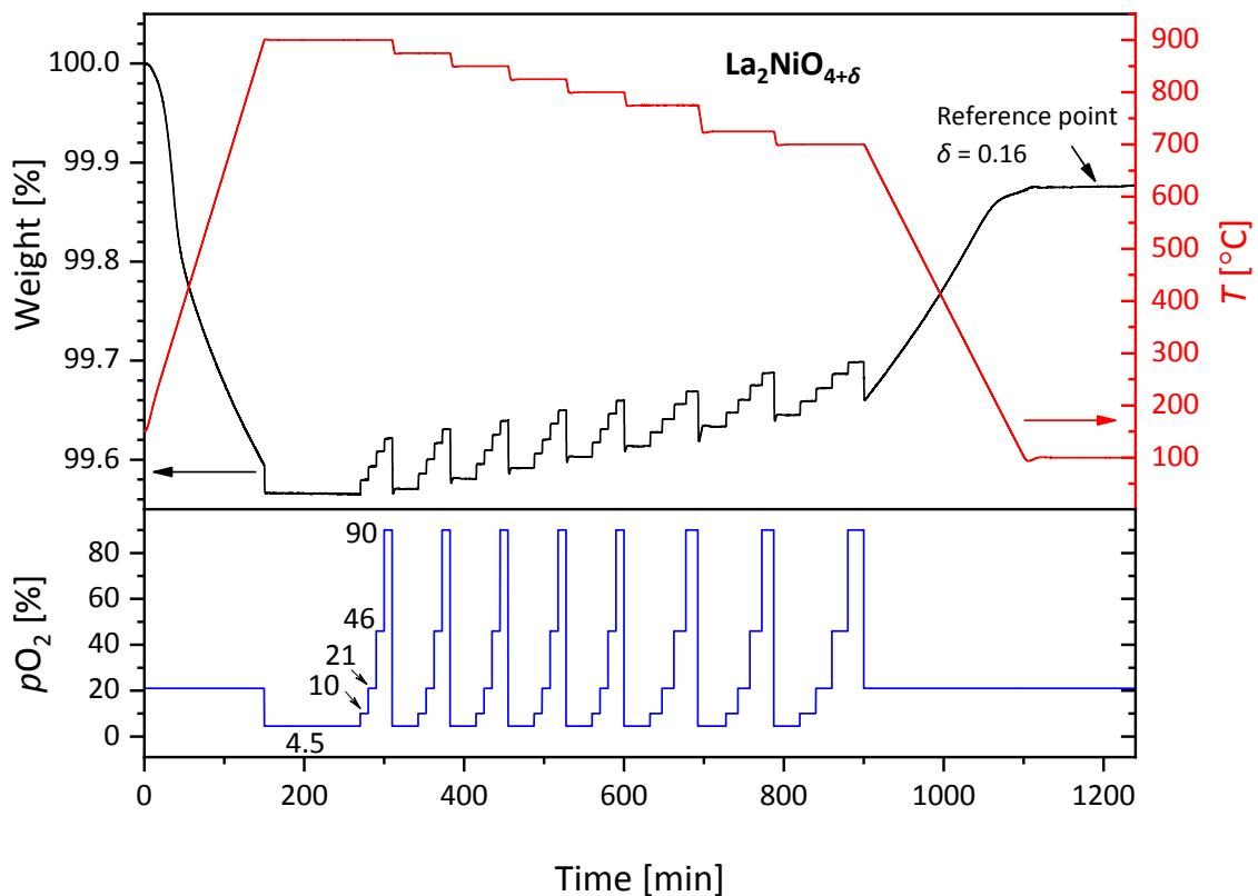
**Figure S10** — Weight loss curve for  $\text{La}_2\text{NiO}_{4+\delta}$  on cooling from 900 °C to 700 °C, with intervals of 25 °C, at different  $p\text{O}_2$  values. The reference point was selected after equilibration for 3 h at  $T = 100$  °C and  $p\text{O}_2 = 0.21$  bar. The corresponding value ( $\delta = 0.16$ ) was determined by reduction in hydrogen (16%  $\text{H}_2/\text{Ar}$ ).
