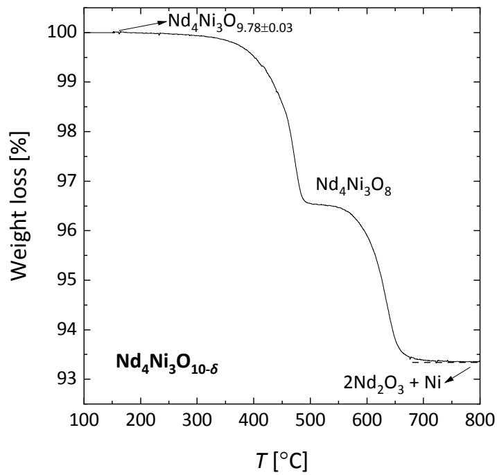
**Figure S9** — Weight loss curve for  $\text{Nd}_4\text{Ni}_3\text{O}_{10-\delta}$  in 16%  $\text{H}_2/\text{Ar}$ .
