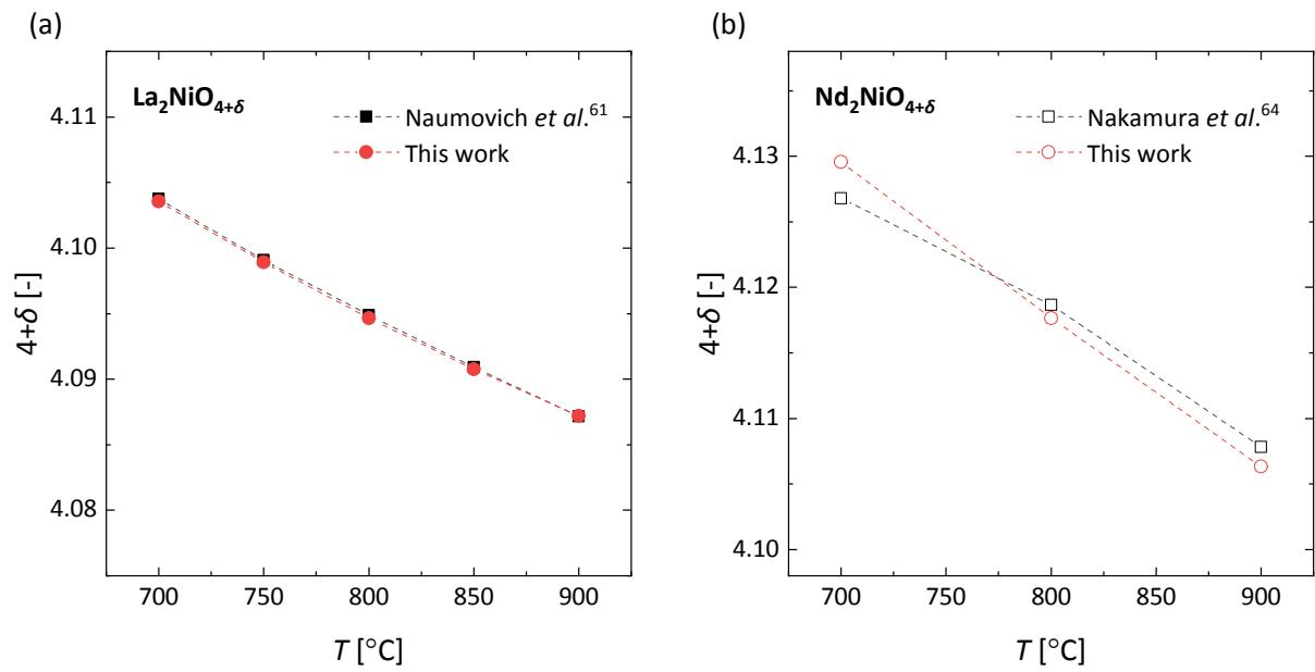
**Figure S15** — Comparison of the temperature dependence of the oxygen stoichiometry measured, in air, for (a)  $\text{La}_2\text{NiO}_{4+\delta}$  and (b)  $\text{Nd}_2\text{NiO}_{4+\delta}$  with corresponding data reported in literature.
