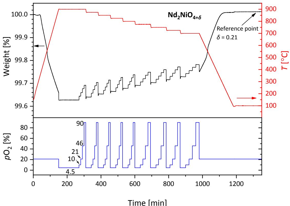
**Figure S11** — Weight loss curve for  $\text{Nd}_2\text{NiO}_{4+\delta}$  on cooling from 900 °C to 700 °C, with intervals of 25 °C, at different  $p\text{O}_2$  values. The reference point was selected after equilibration for 3 h at  $T = 100$  °C and  $p\text{O}_2 = 0.21$  bar. The corresponding value ( $\delta = 0.21$ ) was determined by reduction in hydrogen (16%  $\text{H}_2/\text{Ar}$ ).
