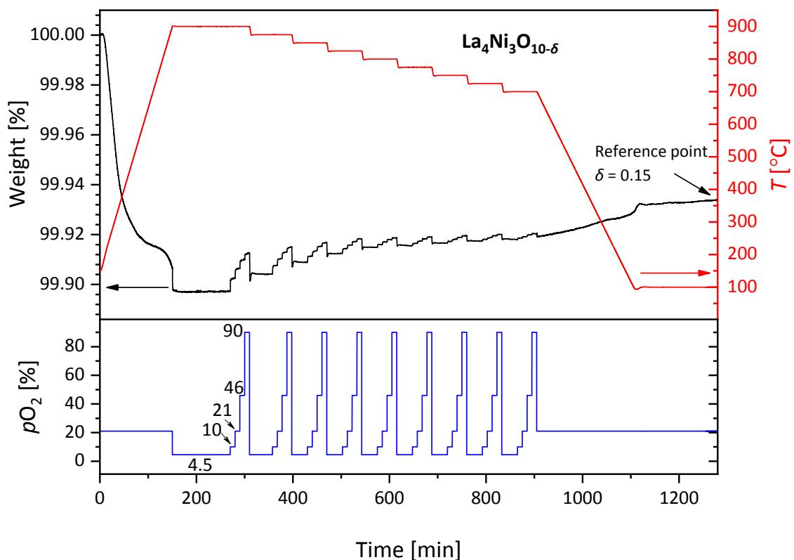
**Figure S13** — Weight loss curve for La<sub>4</sub>Ni<sub>3</sub>O<sub>10- $\delta$</sub>  on cooling from 900  $^{\circ}$ C to 700  $^{\circ}$ C, with intervals of 25  $^{\circ}$ C, at different  $pO_2$  values. The reference point was selected after equilibration for 3 h at  $T = 100$   $^{\circ}$ C and  $pO_2 = 0.21$  bar. The corresponding value ( $\delta = 0.15$ ) was determined by reduction in hydrogen (16% H<sub>2</sub>/Ar).
