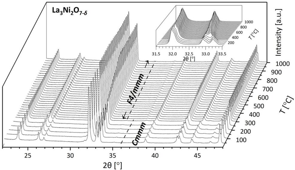
**Figure S3** — *In situ* HT-XRD patterns for  $\text{La}_3\text{Ni}_2\text{O}_{7-\delta}$  (powder) between  $22^\circ$  and  $48^\circ$  recorded in air from  $40^\circ\text{C}$  to  $1000^\circ\text{C}$ , showing the transition from orthorhombic  $Cmmm$  to tetragonal  $F4/mmm$  at approx.  $300^\circ\text{C}$ . The inset shows a magnification of the peaks between  $31.5^\circ - 33.5^\circ$ .
