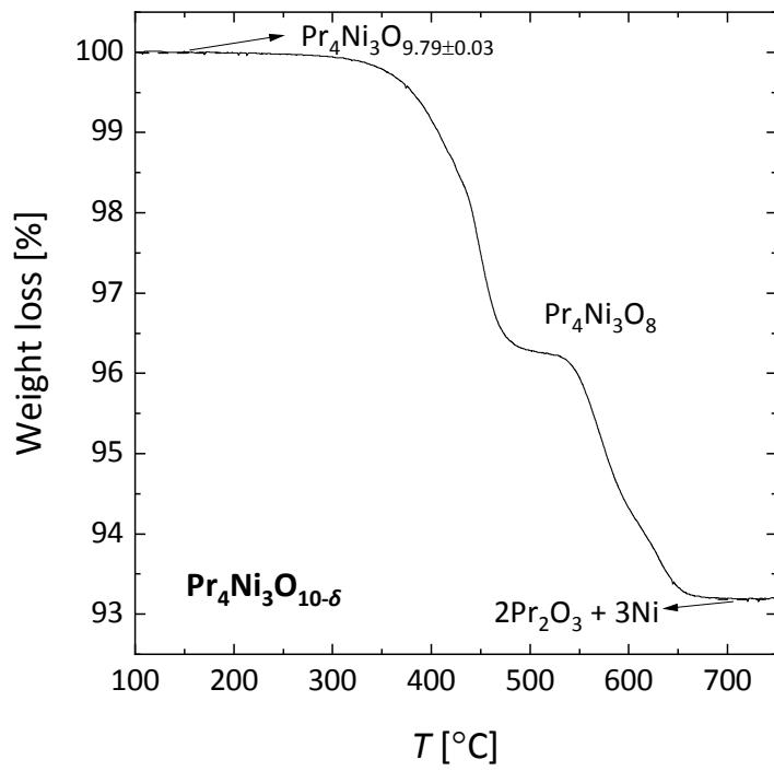
**Figure S8** — Weight loss curve for  $\text{Pr}_4\text{Ni}_3\text{O}_{10-\delta}$  in 16%  $\text{H}_2/\text{Ar}$ .
