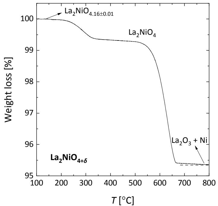
**Figure S6** —Weight loss curve for  $\text{La}_2\text{NiO}_{4+\delta}$  in 16%  $\text{H}_2/\text{Ar}$ .
