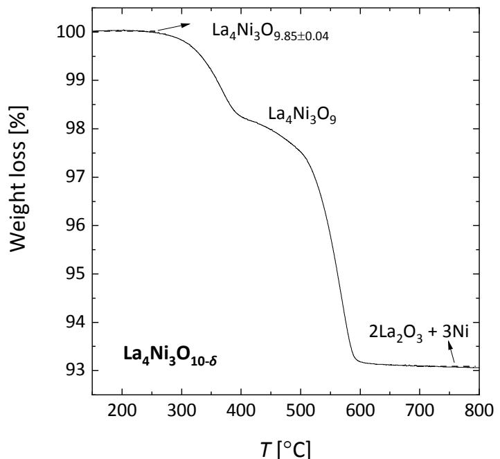
**Figure S7** — Weight loss curve for  $\text{La}_4\text{Ni}_3\text{O}_{10-\delta}$  in 16%  $\text{H}_2/\text{Ar}$ .
