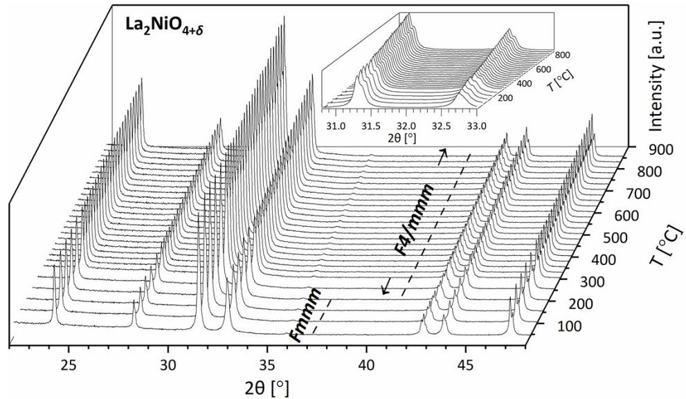
**Figure S1** — *In situ* HT-XRD patterns for  $\text{La}_2\text{NiO}_{4+\delta}$  (powder) between  $22^\circ$  and  $48^\circ$  recorded in air from  $40^\circ\text{C}$  to  $1000^\circ\text{C}$ , showing a phase transition from orthorhombic  $Fm\bar{m}m$  to tetragonal  $F4/m\bar{m}m$  at approx.  $175^\circ\text{C}$ . The inset shows a magnification of the peaks between  $30.8^\circ - 33.0^\circ$ .
