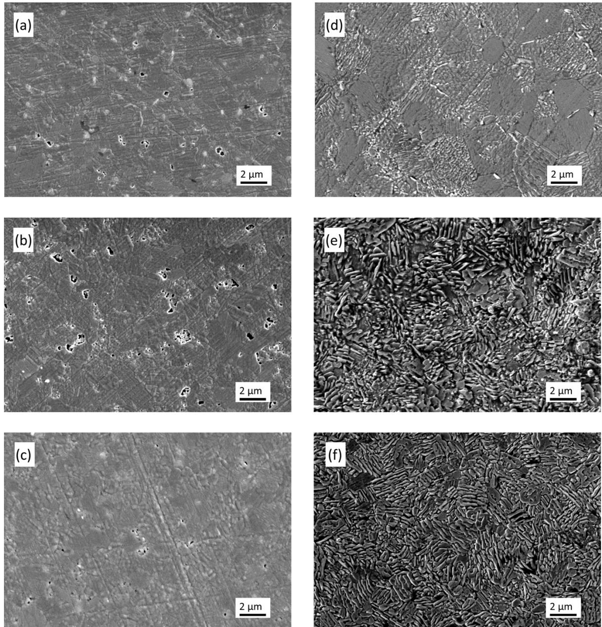
**Figure S16**—SEM images of (a, b, c) sintered polished samples, after thermal etching at 1000 °C for 2 h in air, with those of (d, e, f) samples obtained after the ECR experiments for (a, d)  $\text{La}_2\text{NiO}_{4+\delta}$ , (b, e)  $\text{La}_3\text{Ni}_2\text{O}_{7-\delta}$  and (c, f)  $\text{La}_4\text{Ni}_3\text{O}_{10-\delta}$ .
