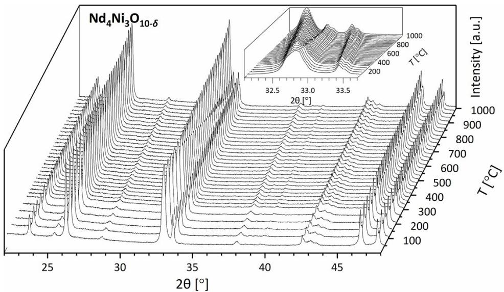
**Figure S5** — *In situ* HT-XRD patterns for  $\text{Nd}_4\text{Ni}_3\text{O}_{10-\delta}$  (powder) between  $22^\circ$  and  $48^\circ$  recorded in air from  $40^\circ\text{C}$  to  $1000^\circ\text{C}$ . The structure remains monoclinic  $P2_1/a$  up to  $1000^\circ\text{C}$ . The inset shows a magnification of the peaks between  $32.1^\circ - 33.7^\circ$ .
