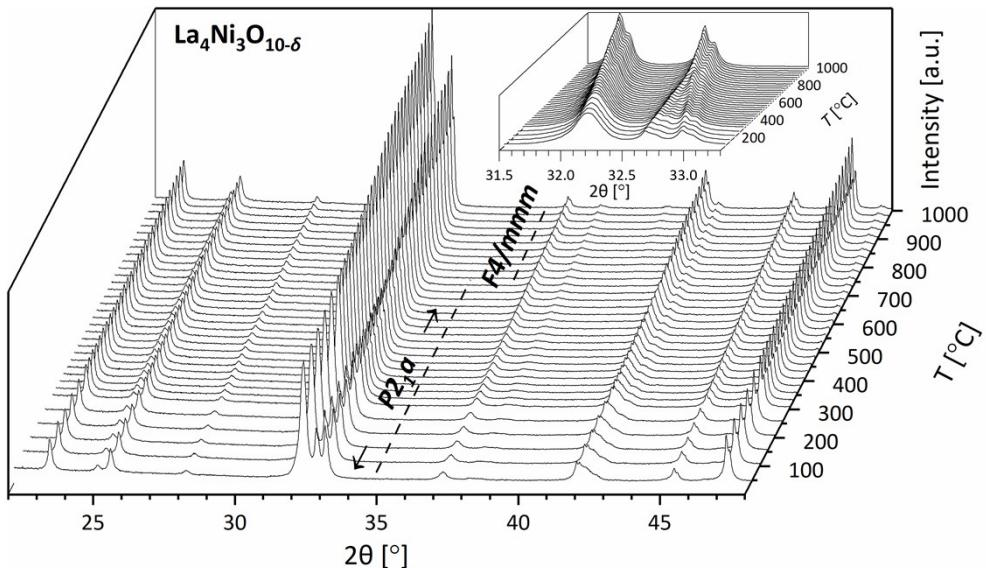
**Figure S4** — *In situ* HT-XRD patterns for  $\text{La}_4\text{Ni}_3\text{O}_{10-\delta}$  (powder) between  $22^\circ$  and  $48^\circ$  recorded in air from  $40^\circ\text{C}$  to  $1000^\circ\text{C}$ , showing the transition from monoclinic  $P2_1a$  to tetragonal  $F4/mmm$  at approx.  $750^\circ\text{C}$ . The inset shows a magnification of the peaks between  $31.5^\circ - 33.3^\circ$ .
