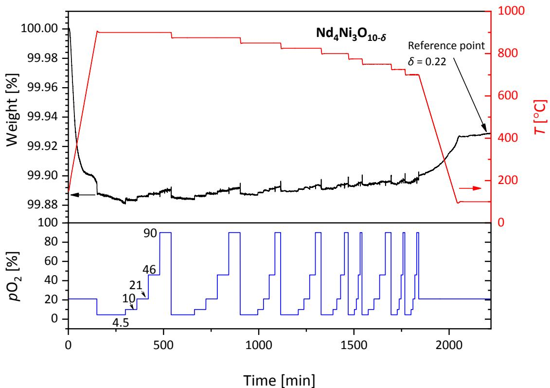
**Figure S14** — Weight loss curve for  $\text{Nd}_4\text{Ni}_3\text{O}_{10-\delta}$  on cooling from 900 °C to 700 °C, with intervals of 25 °C, at different  $p\text{O}_2$  values. The reference point was selected after equilibration for 3 h at  $T=100$  °C and  $p\text{O}_2=0.21$  bar. The corresponding value ( $\delta=0.15$ ) was determined by reduction in hydrogen (16%  $\text{H}_2/\text{Ar}$ ).
