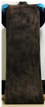
**Figure S19.** Digital photo of a large piece of CuO-CeO<sub>2</sub>/fibrillated para-aramid nonwoven.
