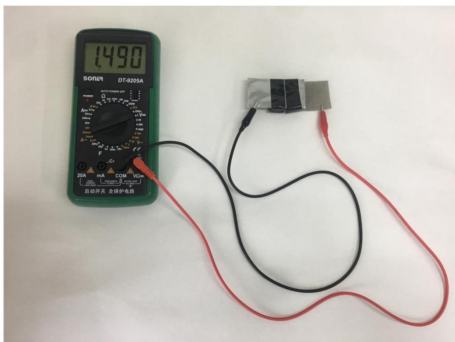
**Figure S21.** Open circuit voltage of the all-solid-state Zn-air batteries with CoFe@NC/CC as air-cathodes.
