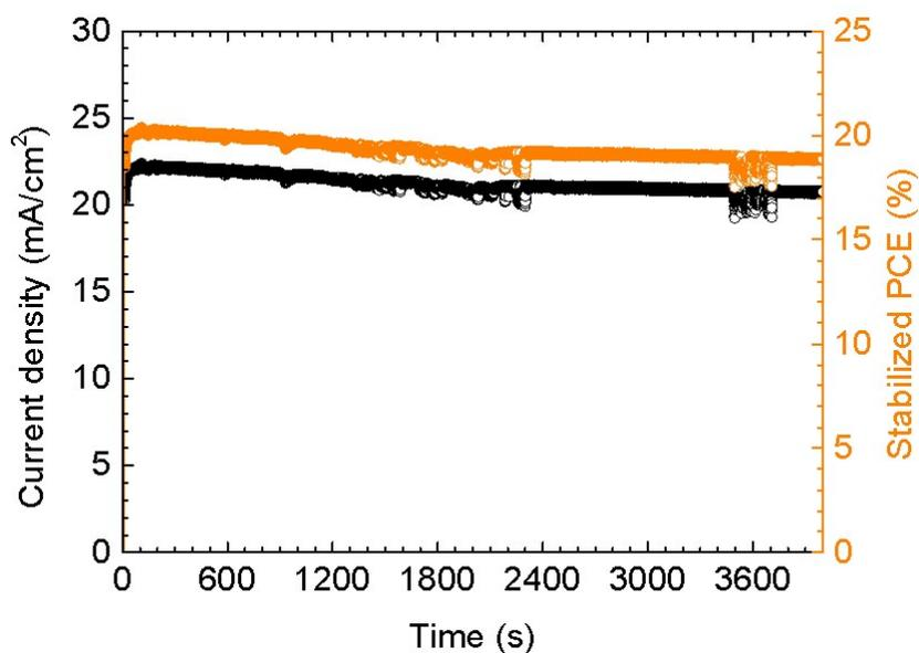
**Figure S6.** The steady-state PCE and current density at maximum power voltage for PSC (active area = 0.125 cm<sup>2</sup>) employing the (FAPbI<sub>3</sub>)<sub>0.95</sub>(CsPbBr<sub>3</sub>)<sub>0.05</sub> film formed from the 0.5 M DMPU-contained solution.
