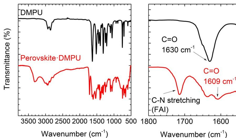
**Figure S1.** FT-IR spectra of the as-formed perovskite-DMPU powder (red line) and DMPU (black line) as reference. C-N stretching is related to FAI.
