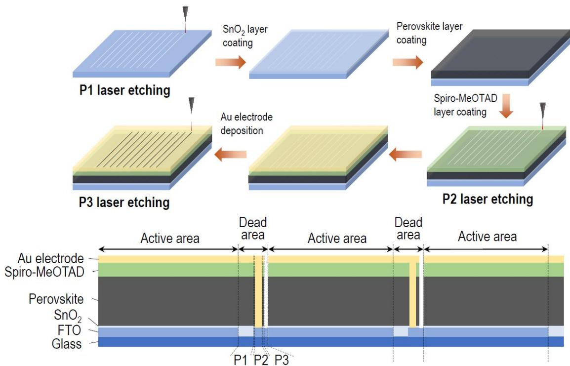
**Figure S7.** Schematic illustration of the fabrication process (top panel) and cross-sectional structure (bottom panel) for a perovskite solar module. P1, P2 and P3 etching was performed by a laser scriber.
