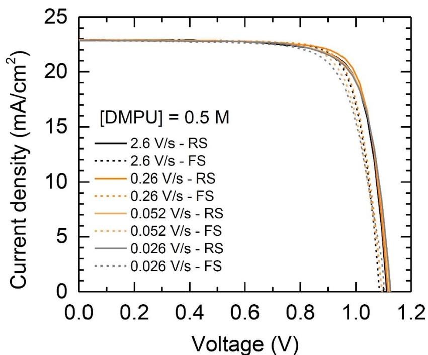
**Figure S5.** Scan-rate and direction dependent J-V curves of PSC employing a piece of the large-area perovskite film formed from the D-bar coating the 0.5 M DMPU-contained precursor solution. The device was measured under AM 1.5G 1 sun illumination with active area of 0.125 cm<sup>2</sup>. RS and FS stand for reverse scan and forward scan, respectively.
