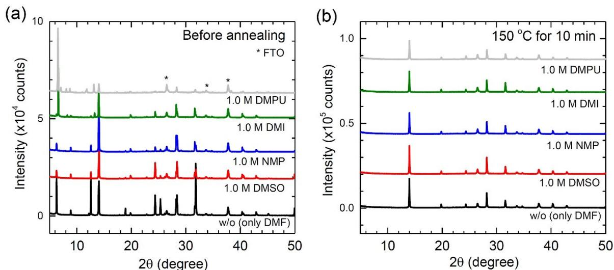
**Figure S2.** XRD patterns of (a) as-deposited and (b) 150 °C-annealed films formed from the air-knife-assisted D-bar coating using the Lewis base (DMSO, NMP, DMI or DMPU) contained precursor solution. Concentration of the Lewis base was 1.0 M. The perovskite composition was  $(\text{FAPbI}_3)_{0.95}(\text{CsPbBr}_3)_{0.05}$ . DMF was used as solvent for the precursor solution.
