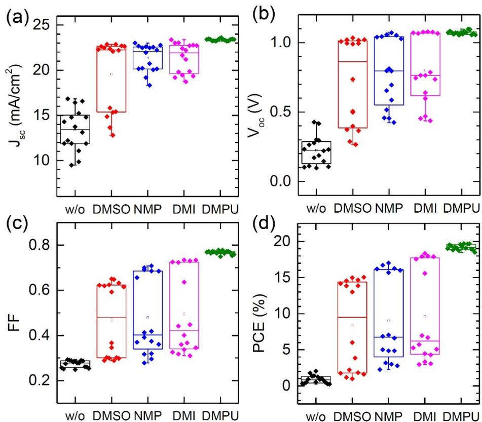
**Figure S4.** Statistical photovoltaic parameters of (a)  $J_{sc}$ , (b)  $V_{oc}$ , (c) FF and (d) PCE for PSCs employing the  $(FAPbI_3)_{0.95}(CsPbBr_3)_{0.05}$  perovskite films formed from the air-knife-assisted D-bar coating using the Lewis base (DMSO, NMP, DMI or DMPU) contained precursor solutions. The Lewis base concentration was 0.5 M. The reverse scanned data are presented.
