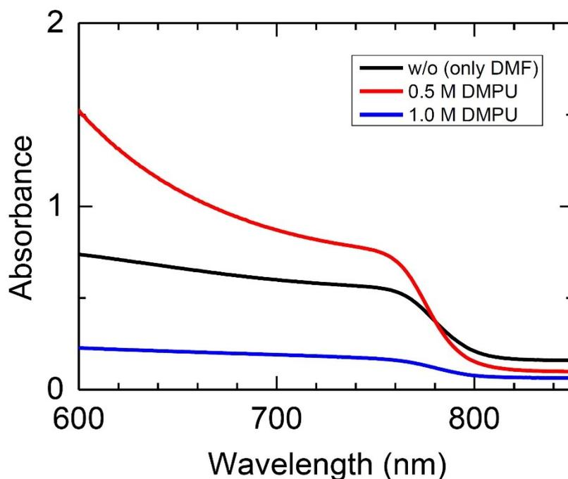
**Figure S3.** Optical absorption spectra of the 150 °C-annealed perovskite films formed from the DMPU-contained precursor solution with different DMPU concentration of 0.5 M and 1.0 M. DMF was used as a solvent for the precursor solution. Perovskite  $(\text{FAPbI}_3)_{0.95}(\text{CsPbBr}_3)_{0.05}$  films were coated on the  $\text{SnO}_2$ -coated FTO substrates by the air-knife-assisted D-bar coating.
