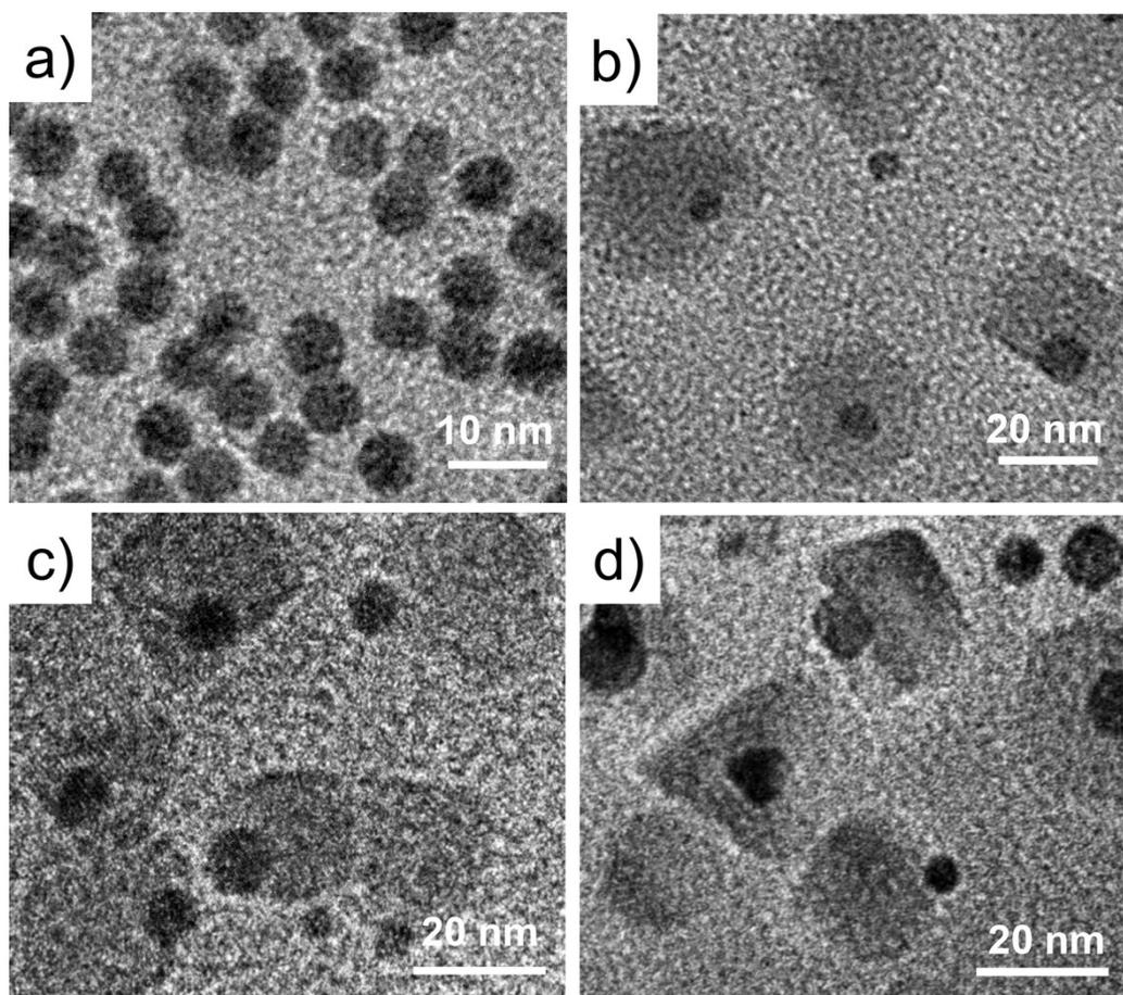
**Fig. S1.** TEM micrographs of (a) Au NPs, (b) Au-Fe<sub>3</sub>O<sub>4</sub> heterodimerics, (c) Au-Fe<sub>3</sub>O<sub>4</sub>@PDA, and (d) Au-Fe<sub>3</sub>O<sub>4</sub>@PDA-PEG, respectively.
