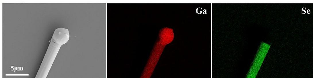
**Figure S1** FESEM image and the corresponding element mapping of a single GaSe microbelt with a spherical particle on the tip.
