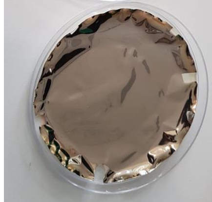
Figure S4. Silver as a reflective layer. Photograph of a sample with 150 nm Ag layer deposited on CNF paper, showing yellowish appearance.
