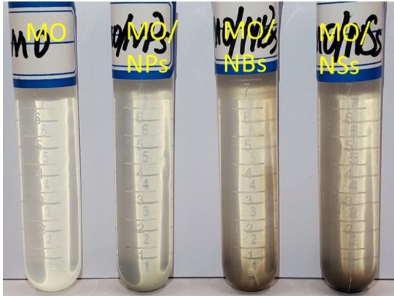
Figure S2. Image of pure oil and 0.00wt% nanofluids after standing for three months
