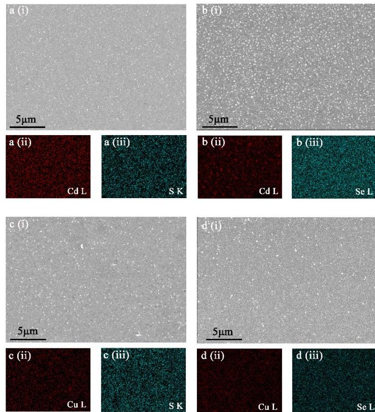
**Figure 3S** SEM images and EDS mapping of CdS (a), CdSe (b),  $\text{Cu}_2\text{S}$  (c) and  $\text{Cu}_2\text{Se}$  (d) thin film.
