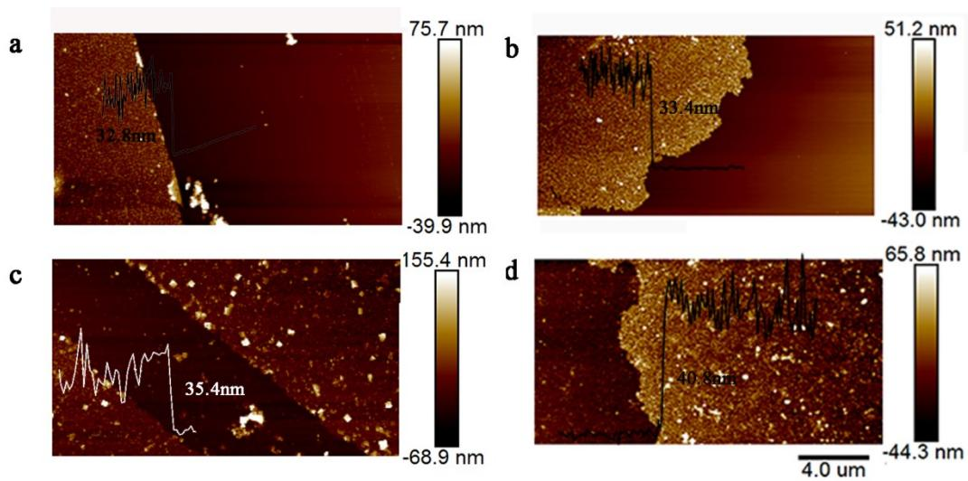
**Figure 4S** The height of as-prepared CdS(a), CdSe(b), Cu<sub>2</sub>S(c) and Cu<sub>2</sub>Se(d) thin films on sapphires when applying 17.5nm Ag thin films as precursors.
