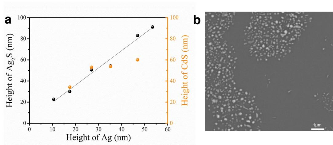
**Figure 2S** (a)the plot about the relation among Ag thin films, as-prepared  $\text{Ag}_2\text{S}$  and CdS. (b) SEM image of CdS when the thickness of silver thin film is less than 10nm
