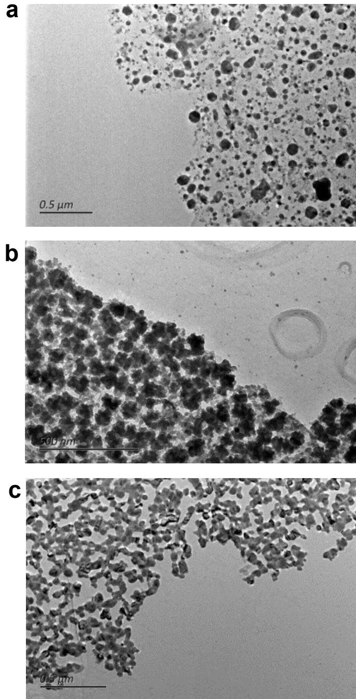
**Figure 1S** (a) the  $\text{Ag}_2\text{S}$  thin film on  $\text{SiO}_2/\text{Si}$  obtained in the furnace at  $200^\circ\text{C}$  for 2h.
