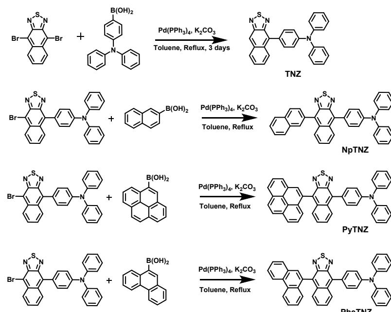
Fig. S1 The synthetic route of TNZ, NpTNZ, PyTNZ and PheTNZ.
