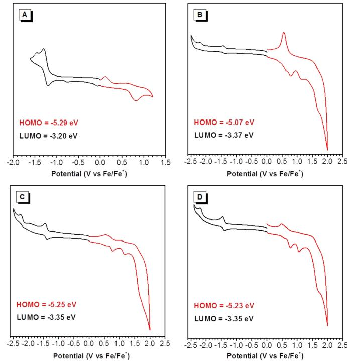
**Fig. S17** Cyclic voltammograms (CV) of these investigated compounds: (A) TNZ, (B) PyTNZ, (C) PheTNZ, (D) NpTNZ.
