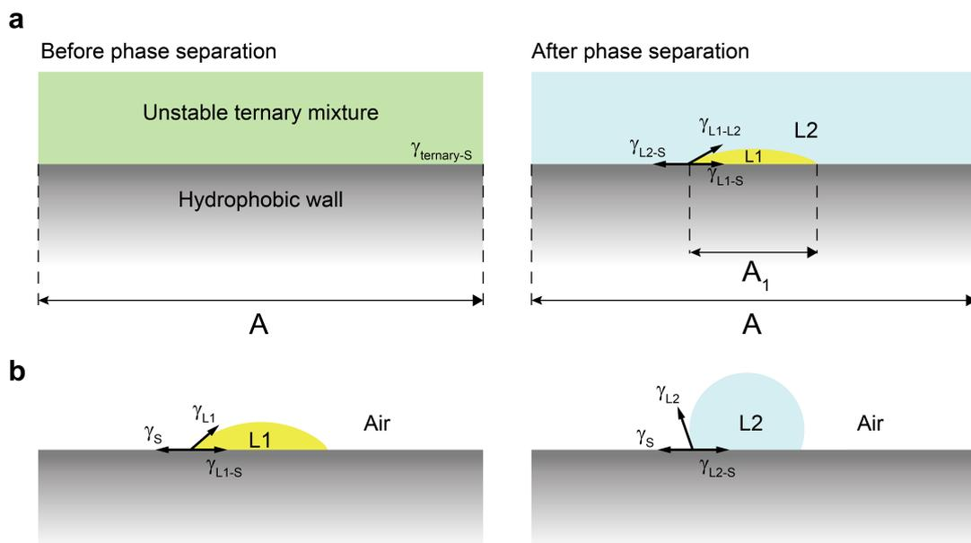
**Figure S2.** a. Schematic showing the interfaces before and after phase separation and their respective interfacial tensions. b. Schematic showing the force balance on oil and water droplets on the hydrophobic substrate surrounded in air.
