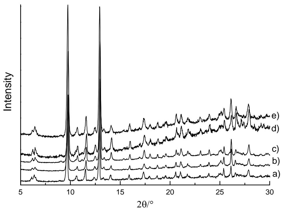
Fig. S7: Powder X-ray patterns of **2** taken after some hours (a), 1 year (b), 2 years (c), 3 years (d), and 4 years (e) after the product was isolated.
