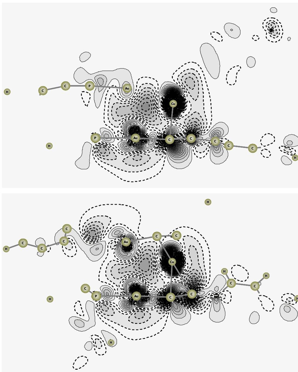
Figure S14. Contour project the deformation of electron density  $\rho(S_0) - \rho(T_1)$  into a plane P–Au–Cu for the complexes **3** (top) and **5** (bottom); optimized  $T_1$  geometry. Solid lines (plus sign) enclose the regions where the electron density is higher in the  $S_0$  state, dashed lines (minus sign) show the regions, in which the electron density is higher in the  $T_1$  state. The atoms located close to the cross-section plane are also shown.
