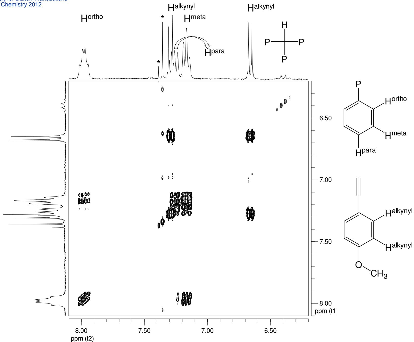
Figure S8. 300 MHz  $^1\text{H}$ - $^1\text{H}$  COSY NMR spectrum of **4** (aromatic range),  $\text{CD}_2\text{Cl}_2$ , ambient temperature. Assignment of the signals is given in the upper part of the figure. Resonances of admixtures are marked with \*.
