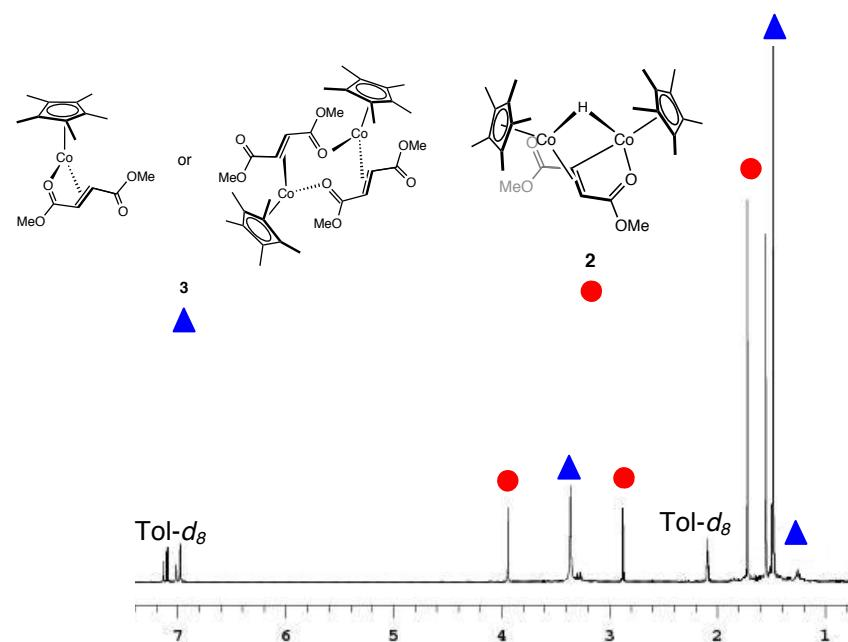
**Figure S18.**  $^1\text{H}$  NMR spectrum of 1:1 reaction of **1** with dimethyl maleate in toluene- $d_8$  at 25 °C.
