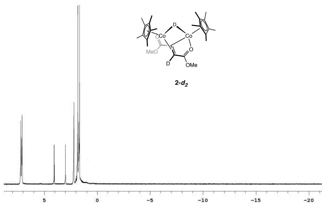
**Figure S3.** <sup>1</sup>H NMR spectrum of **2-d<sub>2</sub>** in toluene-*d*<sub>8</sub> at -45 °C.
