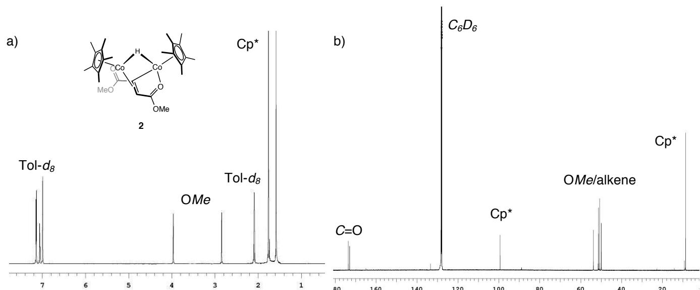
**Figure S1.** a)  $^1\text{H}$  (toluene- $d_8$ ) and b)  $^{13}\text{C}$  NMR spectra (benzene- $d_6$ ) of **2** recorded at 25 °C.
