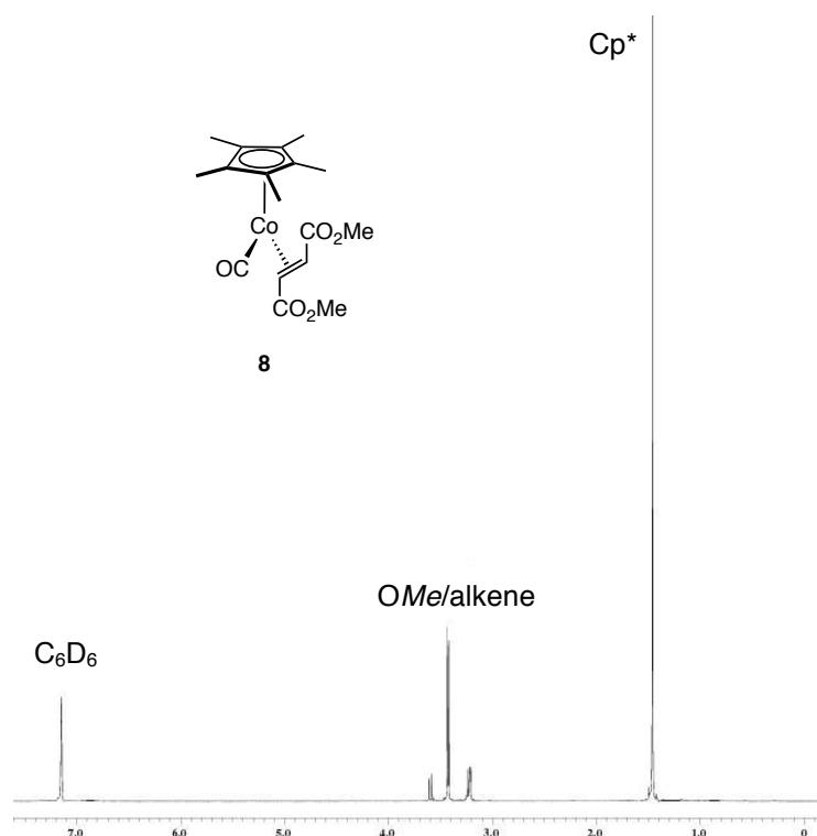
**Figure S15.**  $^1\text{H}$  NMR spectrum of **8** in benzene- $d_6$  at 25 °C.
