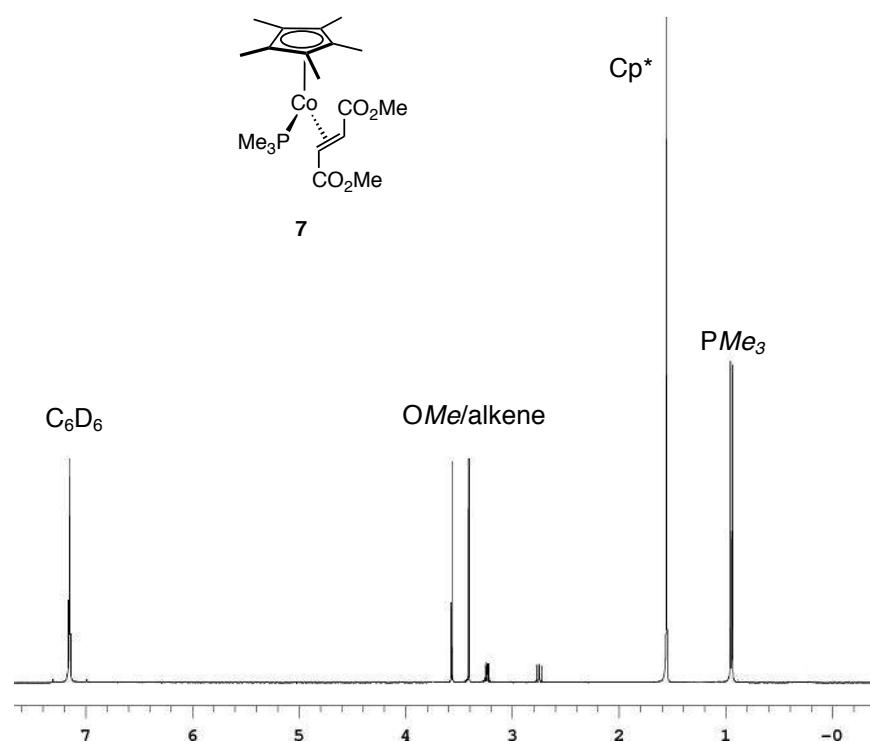
**Figure S13.**  $^1\text{H}$  NMR spectrum of **7** in benzene- $d_6$  at 25 °C.
