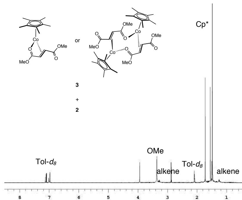
**Figure S5.** <sup>1</sup>H NMR spectrum of a mixture of **2** and **3** in toluene-*d*<sub>8</sub> at 25 °C. Only resonances for **3** are noted; the other peaks belong to **2**.
