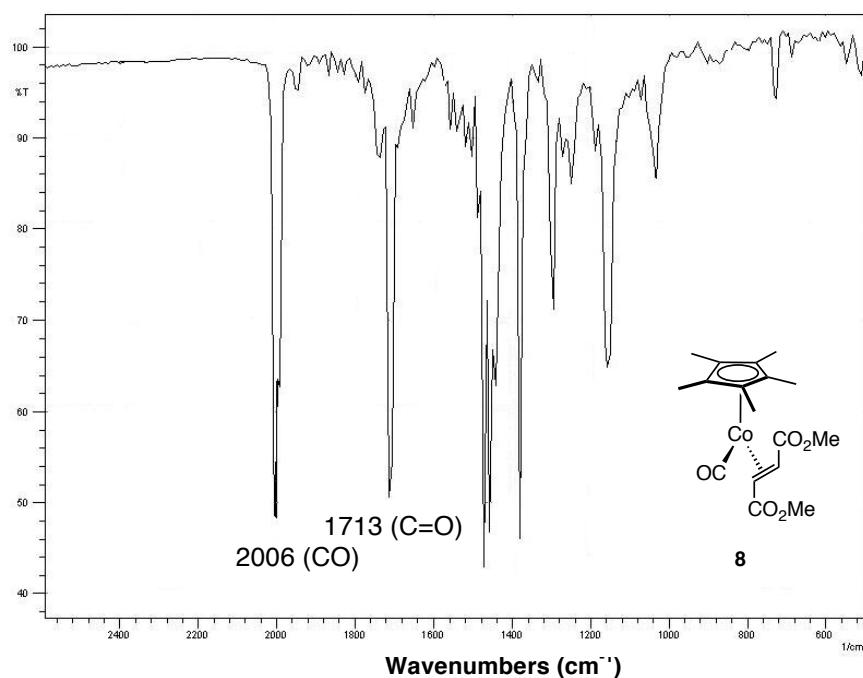
**Figure S17.** Solution IR spectrum of **8** recorded in pentane.
