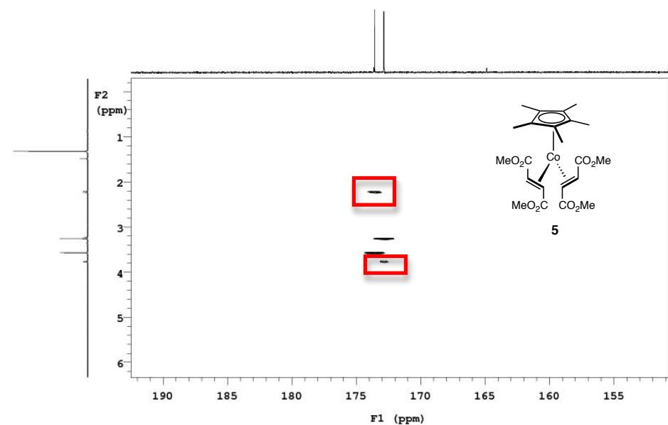
**Figure S8.** HMBC NMR spectrum of **5** in benzene-*d*<sub>6</sub> at 25 °C. Two and three bond coupling of the alkenyl hydrogens to the C=O carbons identify the presence of two vinylic hydrogens (shown in red).
