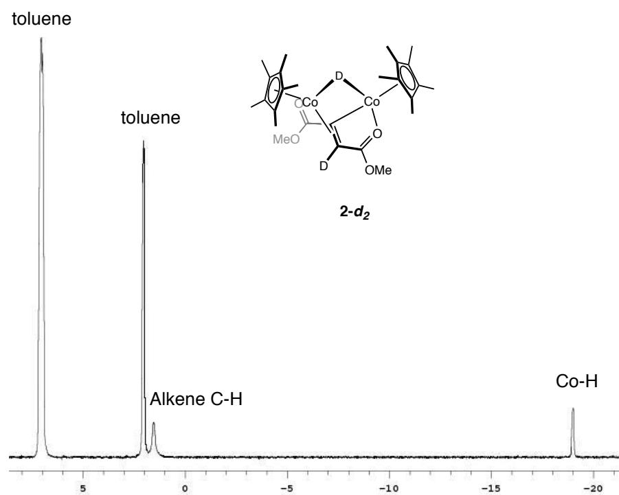
**Figure S4.** <sup>2</sup>H NMR spectrum of **2-d<sub>2</sub>** in toluene at -45 °C.
