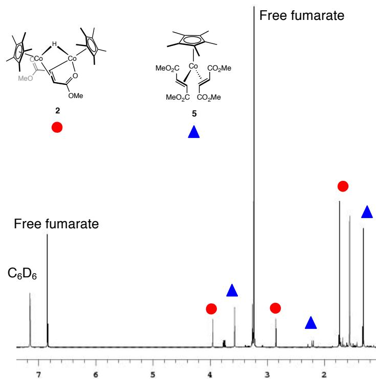
**Figure S12.** <sup>1</sup>H NMR spectrum of addition of excess dimethyl fumarate to a mixture of **3** and **2** after 15 minutes in benzene-*d*<sub>6</sub> at 25 °C.
