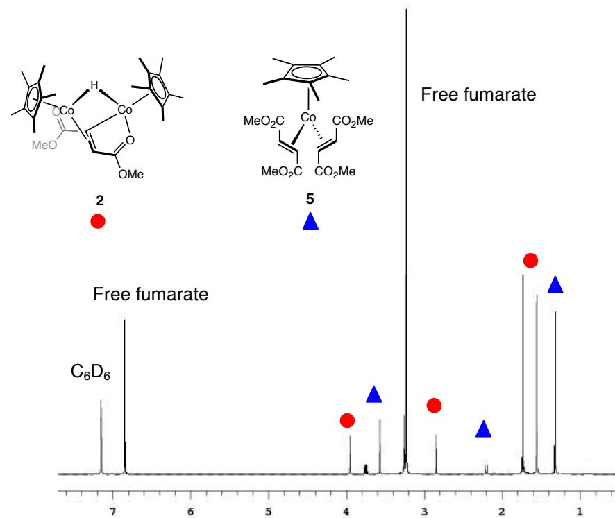
**Figure S9.**  $^1\text{H}$  NMR spectrum of addition of excess dimethyl fumarate to **2** in benzene- $d_6$  at 25 °C.
