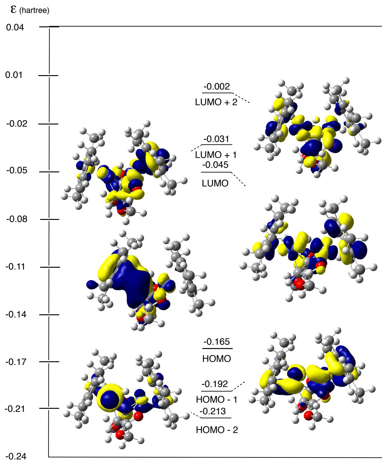
**Figure S20.** Frontier Kohn-Sham molecular orbital diagram of **2** as calculated using the Gaussian 09 program suite. Rendered at an isovalue of  $0.03 \text{ e/}\text{\AA}^3$  ( $\text{e}/\text{\AA}^3 = \text{electrons per Angstrom cubed}$ ). Functional: B3LYP, Basis set: 6-31g(d',p') (C/O/H); LANL2DZ + F polarization (Co).
