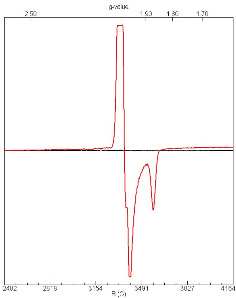
Figure S17. Overlay of the EPR spectra of [\text{Ru}(\text{TPA})(\text{ONO})(\text{NO})](\text{PF}_6)_2 ( 4 , black) and its photoproduct [\text{Ru}(\text{TPA})(\text{ONO})(\text{solv})]^{2+} (red). The spectra were obtained in frozen DMF at 10K.
