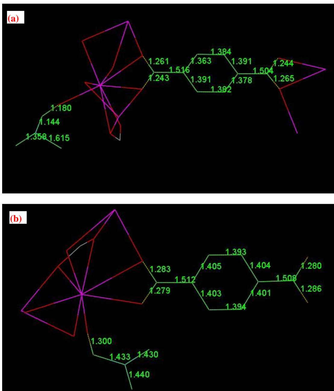
**Figure S2** Bond distances in BDC<sup>2-</sup> and DMF moieties obtained from (a) X-ray single crystal structure analysis at 293 K and (b) crystal structure optimization using the *Materials Studio* program.
