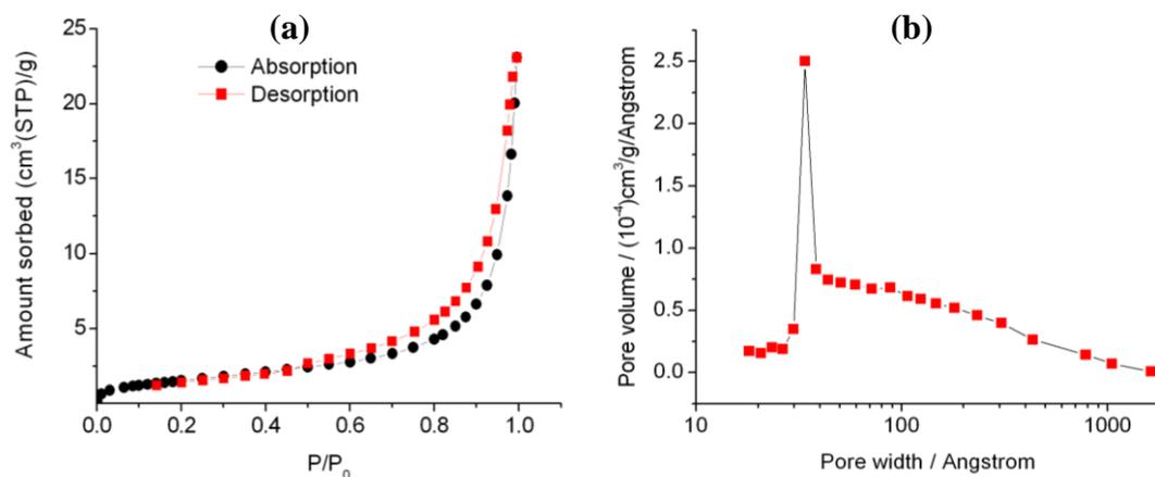
Figure S1 (a) The isotherm for the adsorption and desorption of N<sub>2</sub> on activated **3** at 77 K and (b) pore size distribution.
