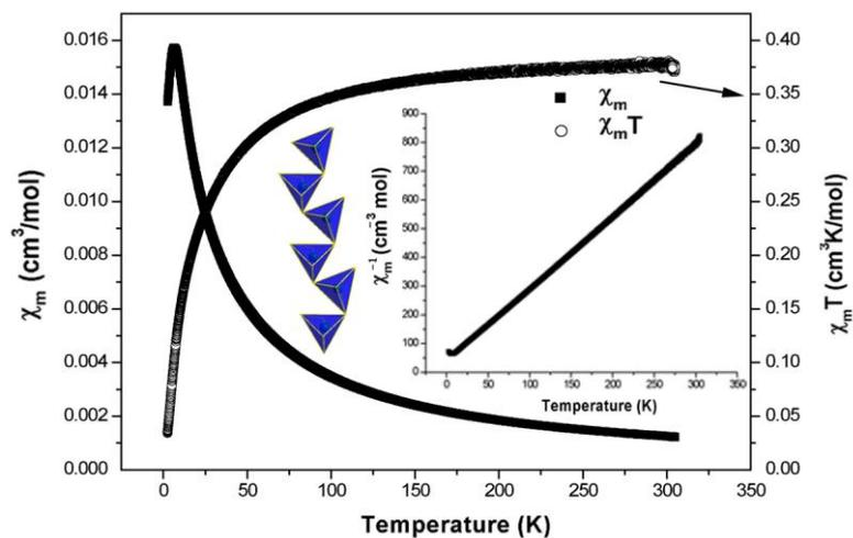
Figure S4. The  $\chi_m$  vs.  $T$  and  $\chi_m T$  vs.  $T$  plots. The insets are  $1/\chi_m$  vs.  $T$  plot and the Cu(1)O<sub>5</sub> polyhedra chain extending along the [100] direction.
