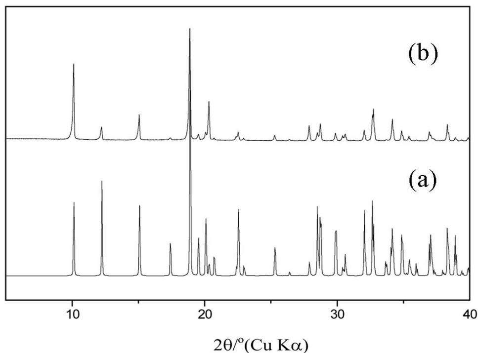
Fig. S1 The simulated XRD pattern (a) and experimental one (b) for compound **1**.
