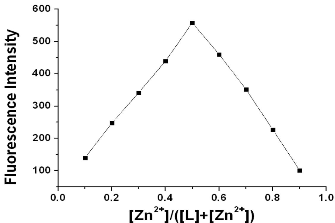
**Fig. S1.** Job plot of a 1:1 complex of L and  $Zn^{2+}$ , where the intensity at 462 nm was plotted against the mole fraction of zinc ions.
