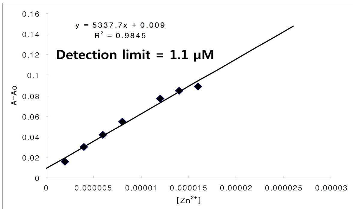
**Fig. S3.** Detection limit of **L** (20 μM) with Zn<sup>2+</sup>.
