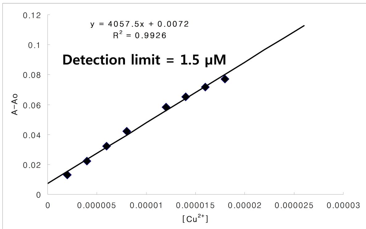
**Fig. S12.** Detection limit of **L** (20  $\mu$ M) with  $Cu^{2+}$ .
