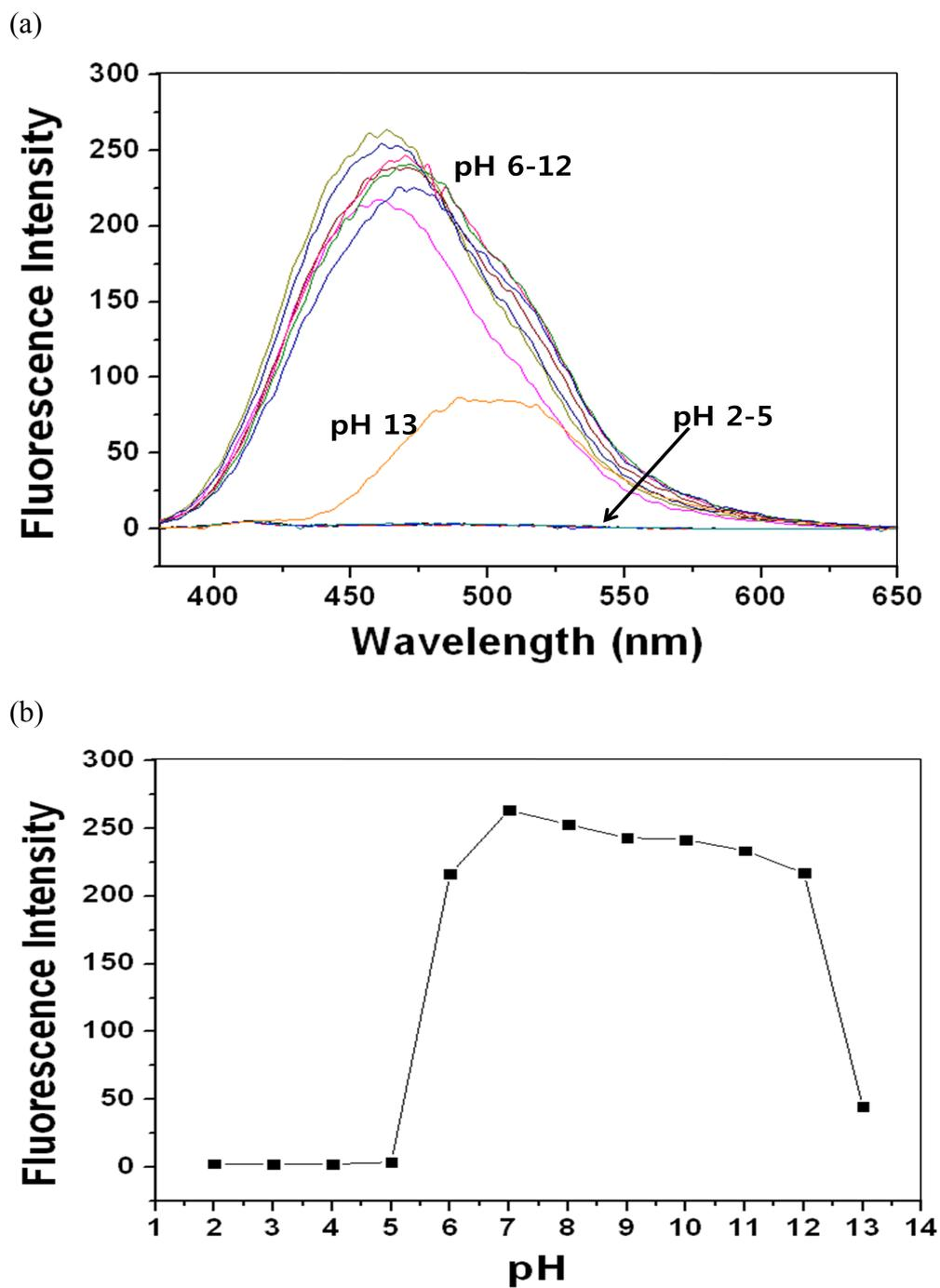
**Fig. S4.** (a) Fluorescence spectra of **L** (10  $\mu$ M) after the addition of zinc ions (1 equiv) at different pH in 10 mM HEPES buffer-CH<sub>3</sub>OH (99:1, v/v). (b) Plot of the fluorescence intensity of **L** at 462 nm against pH.
