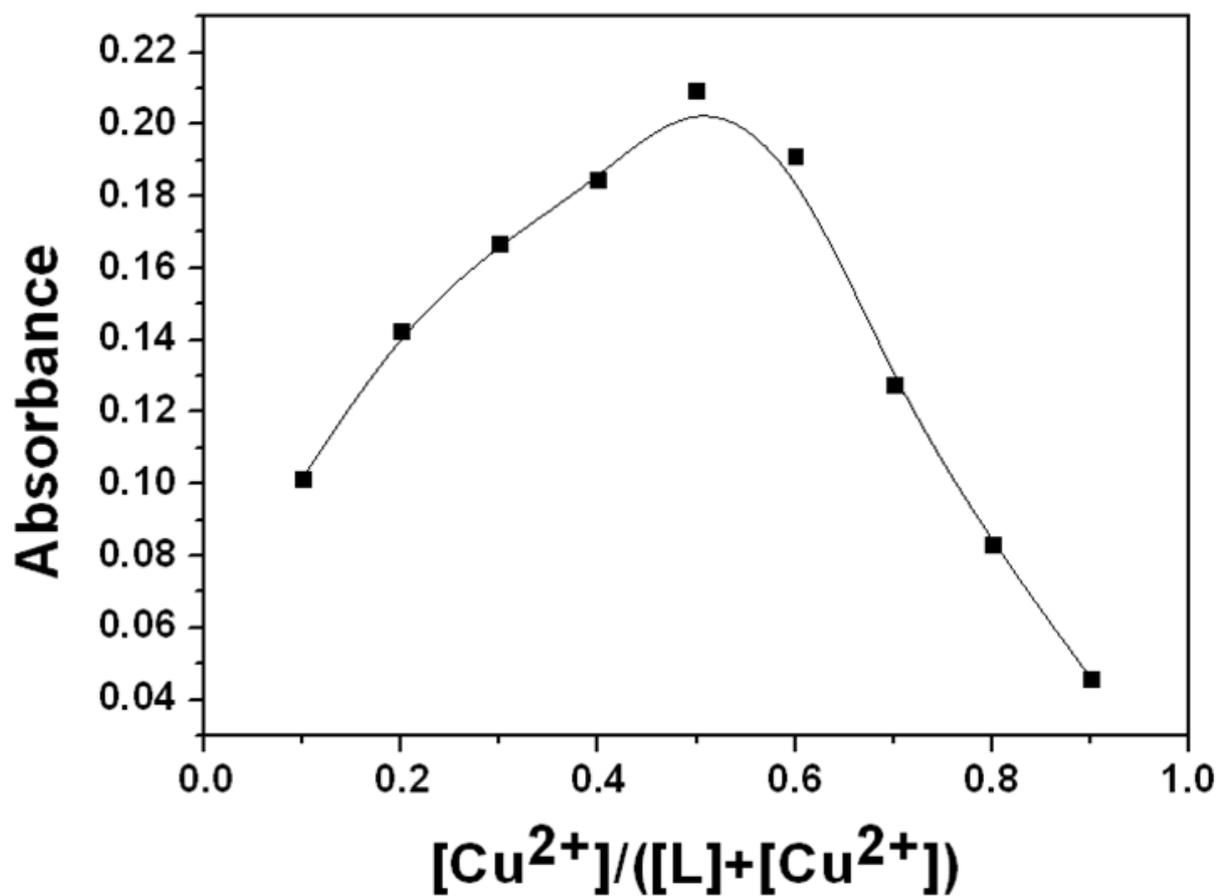
**Fig. S9.** Job plot of a 1:1 complex of L and Cu<sup>2+</sup>, where the absorption at 396 nm was plotted against the mole fraction of copper ions.
