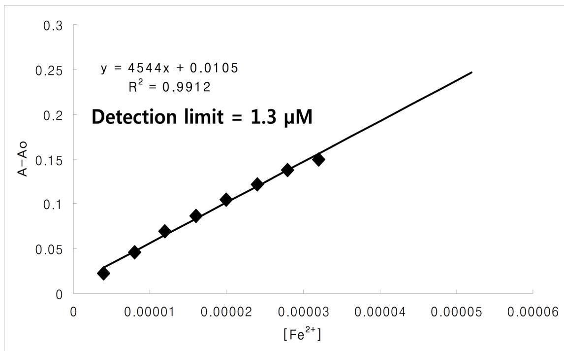
**Fig. S7.** Detection limit of **L** (20 μM) with Fe<sup>2+</sup>.
