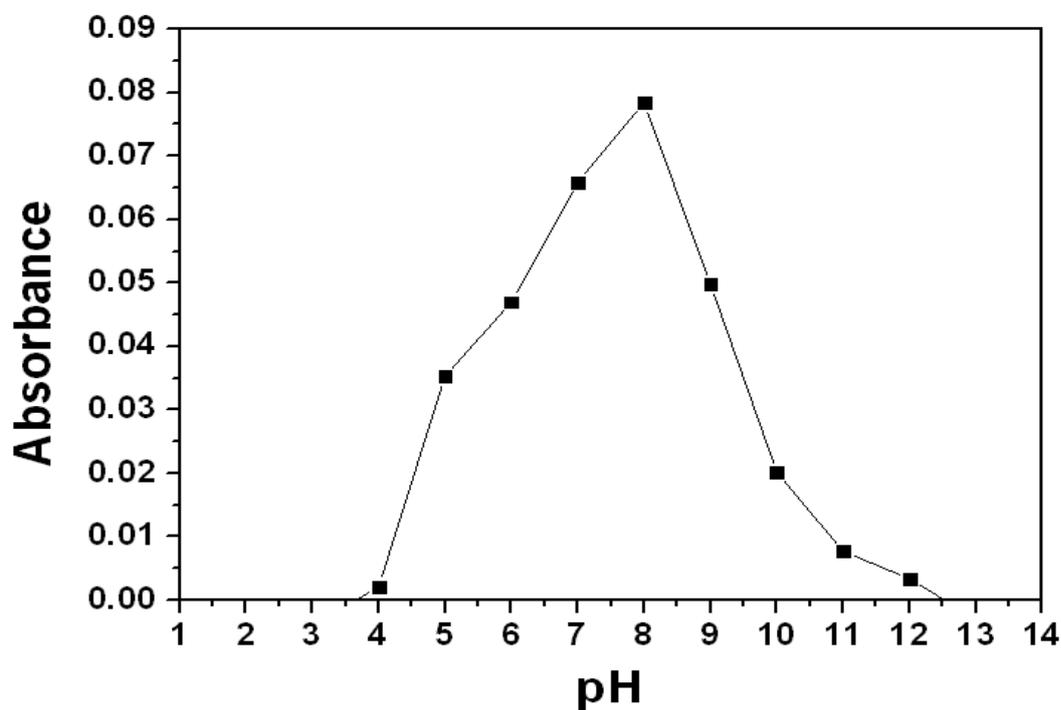
**Fig. S8.** (a) Absorption spectra of **L** (20 μM) after the addition of ferrous ions (2 equiv) in 10 mM HEPES buffer and CH<sub>3</sub>OH (99:1, v/v). (b) Plot of the absorbance of **L** at 509 nm against pH.
