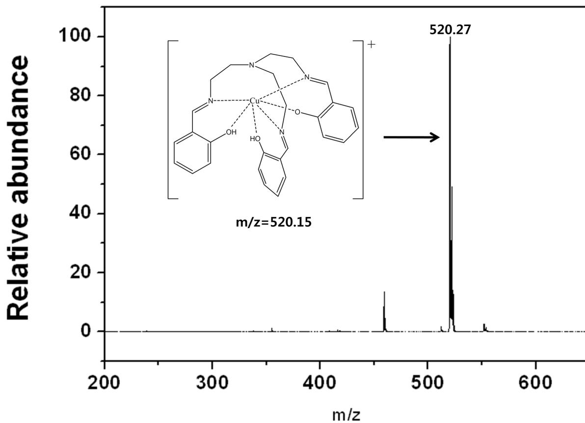
**Fig. S10.** Positive-ion electrospray ionization mass spectrum of **L** upon addition of 1 equiv of  $\text{Cu}^{2+}$  in  $\text{CH}_3\text{OH}$ .
