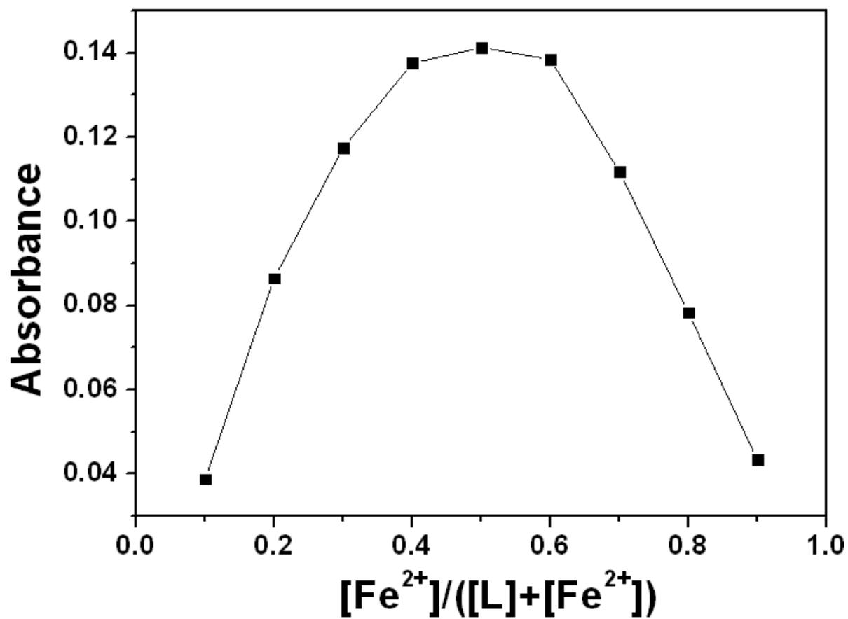
**Fig. S5.** Job plot of a 1:1 complex of L and Fe<sup>2+</sup>, where the absorption at 515 nm was plotted against the mole fraction of ferrous ions.
