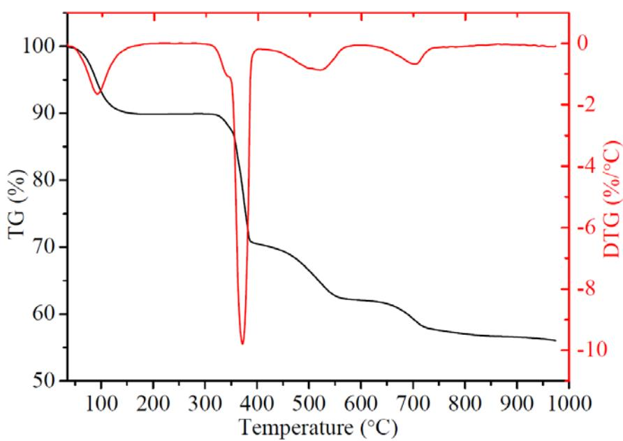
**Fig. S9** TG-DTG curve of  $K_{3n}[Gd(\text{EDTA})(\text{HPO}_3)]_n \cdot 7n\text{H}_2\text{O}$  (**1**)
