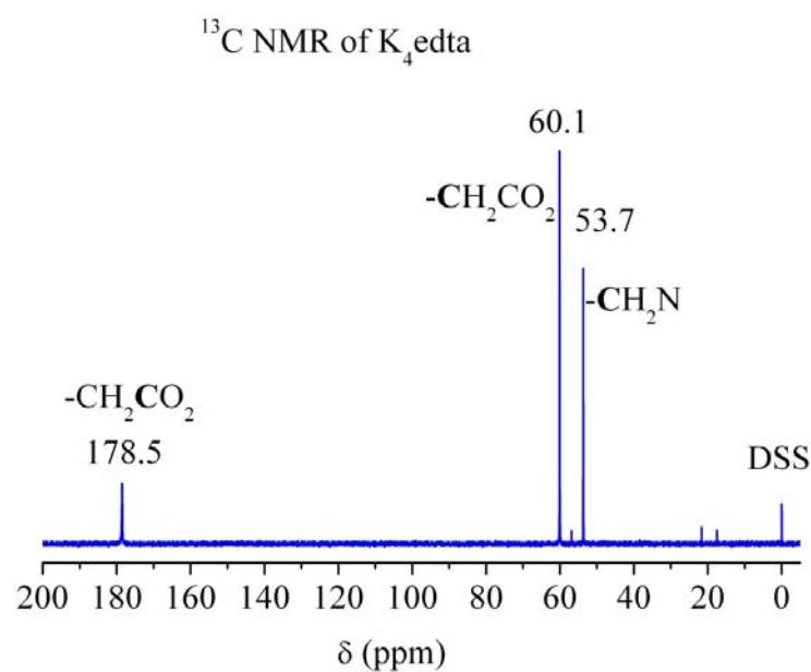
**Fig. S2** Solution <sup>13</sup>C NMR spectrum of K<sub>4</sub>edta
