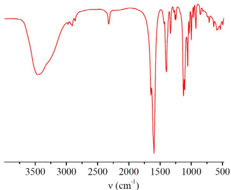
**Fig. S5** IR spectrum of  $\text{K}_{3n}[\text{Gd}(\text{EDTA})(\text{HPO}_3)]_n \cdot 7n\text{H}_2\text{O}$  (**1**)
