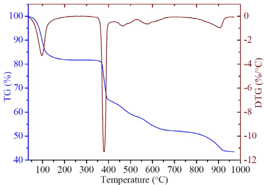
**Fig. S10** TG-DTG curve of  $\text{Na}_6[\text{Gd}_2(\text{EDTA})_2(\text{HPO}_3)_2] \cdot 2.5\text{NaCl} \cdot 21\text{H}_2\text{O}$  (**2**)
