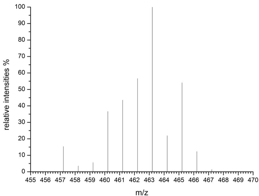
Figure S10 Simulated isotope pattern of  $[\text{RuH}(\text{PNP})]$  **463**.
