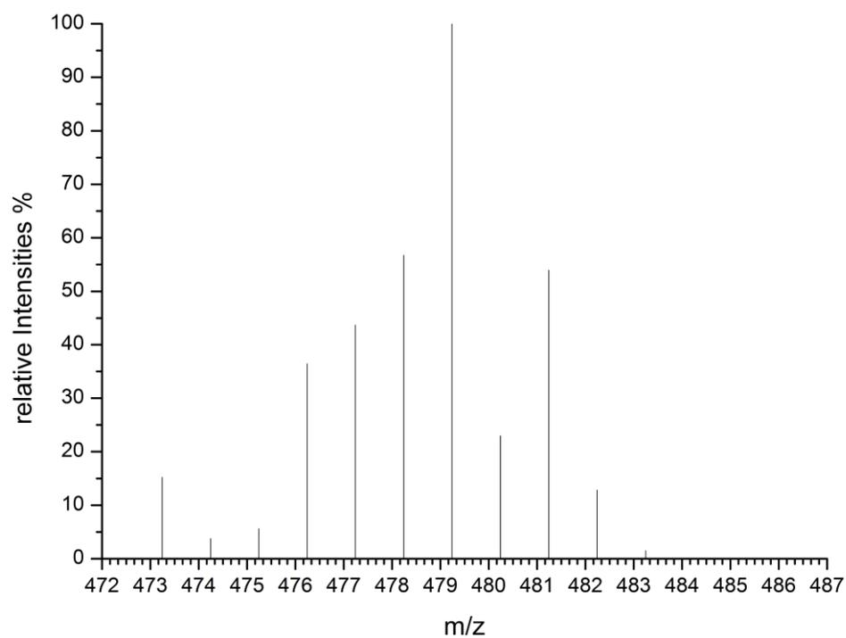
Figure S19 Simulated isotope pattern of fragment  $[\text{RuH}_2(\text{Me-PNP})]$  473 – 482.
