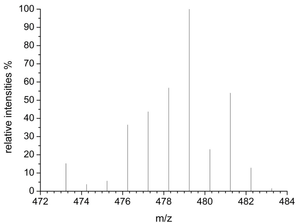
Figure S15 Simulated isotope pattern of  $[\text{RuH}_2(\text{Me-PNP})]$  479.
