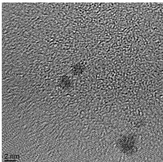
**Figure 3.** HRTEM image of **Ru1Pt1** nanoparticles.
