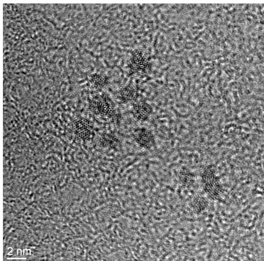
**Figure 5.** HRTEM image of **Ru1Pt4** nanoparticles.
