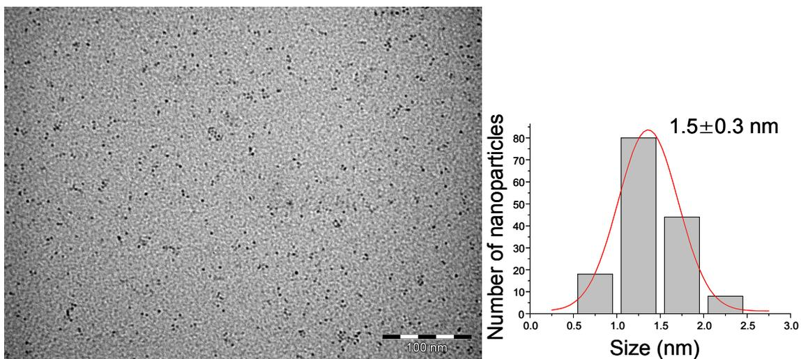
**Figure 17.** TEM image with the corresponding size histogram of **Ru/PPP** nanoparticles after CAL hydrogenation.
