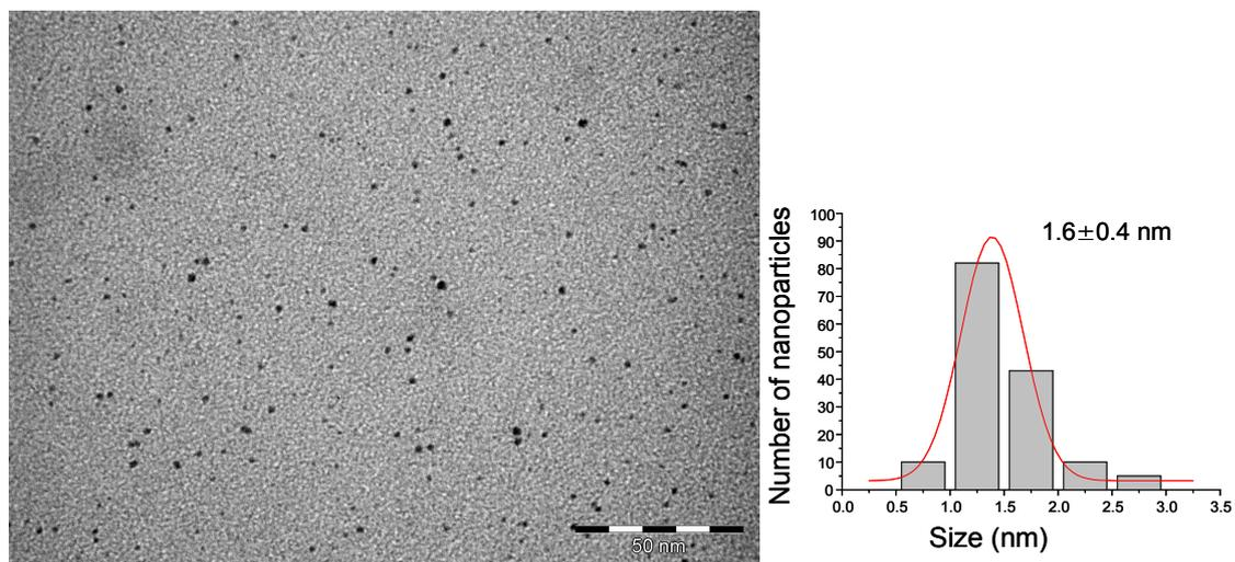
**Figure 13.** TEM image with the corresponding size histogram of **Pt@Ru** nanoparticles after CAL hydrogenation.
