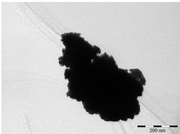
**Figure 1.** TEM micrographs of Pt/PPP particles.
