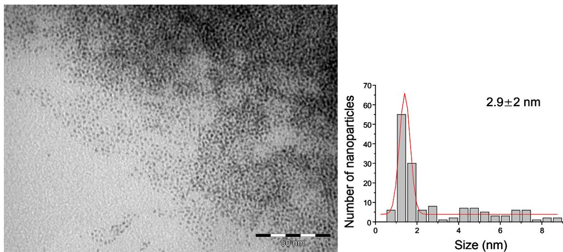
**Figure 12.** TEM image with the corresponding size histogram of **Ru1Pt4** nanoparticles after CAL hydrogenation.
