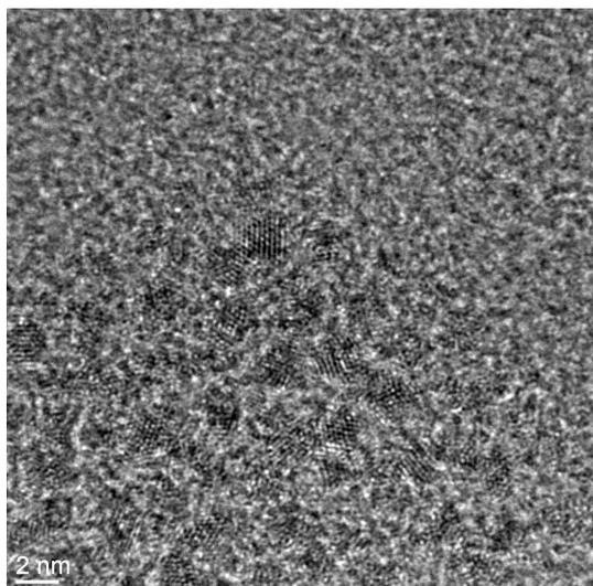
**Figure 6.** HRTEM image of **Pt1Ru1** nanoparticles.
