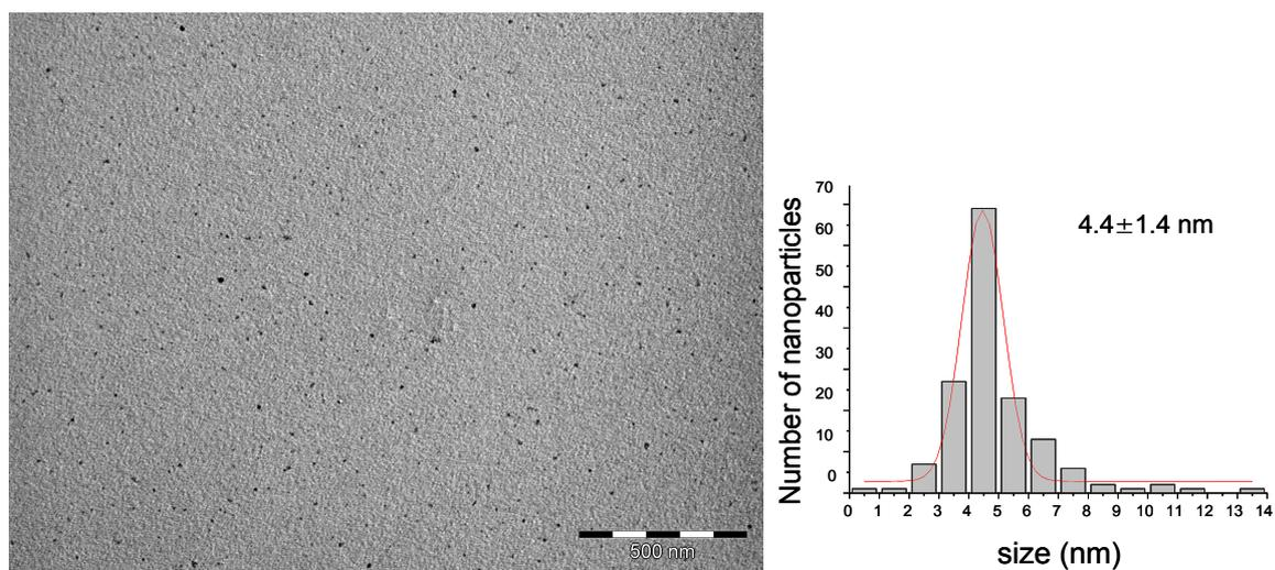
**Figure 10.** TEM image with the corresponding size histogram of **Ru1Pt1** nanoparticles after CAL hydrogenation.
