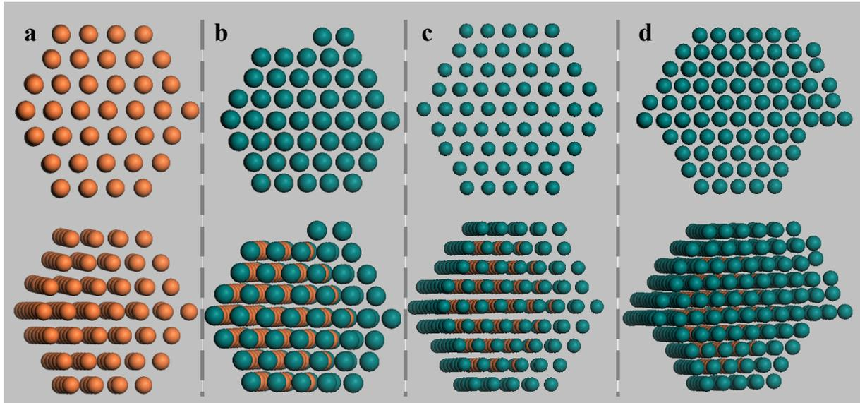
a) Nanoparticle model of monometallic Ru (001) nanoparticles (top along Y axis view and bottom with angles). Model containing 83 atoms (Empirical radius of ruthenium was used in the cluster model,  $1.30 \times 2 \times 6 = 1.56$  nm).
