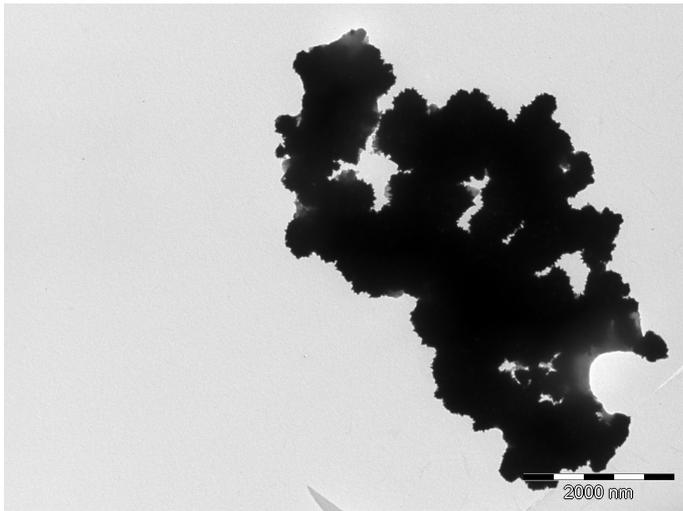
**Figure 18.** TEM image of **Pt/PPP** particles after CAL hydrogenation.
