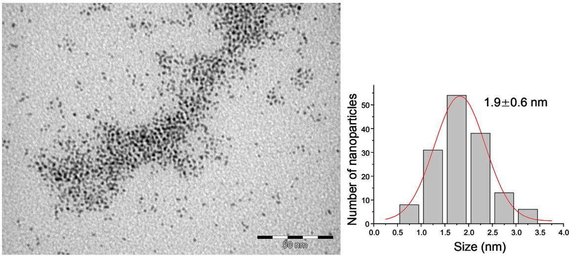
**Figure 19.** TEM image with the corresponding size histogram of **Pt/CO** nanoparticles.
