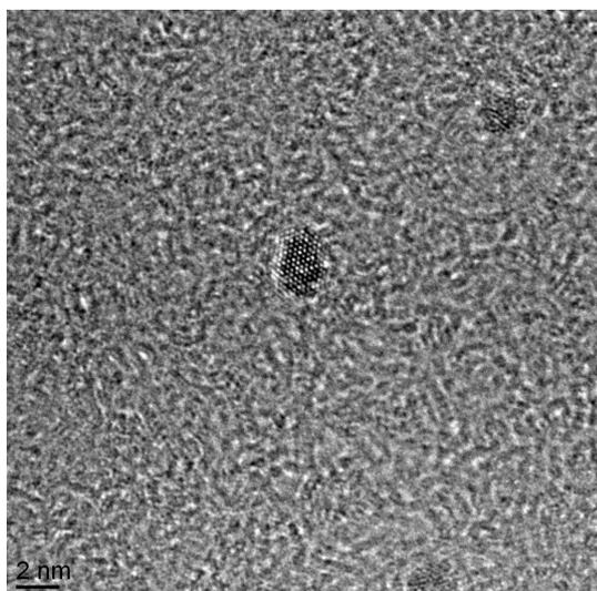
**Figure 4.** HRTEM image of **Ru1Pt2** nanoparticles.
