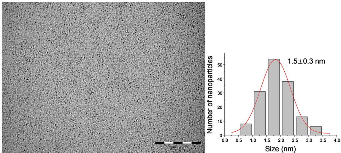
**Figure 16.** TEM image with the corresponding size histogram of **Pt1Ru4** nanoparticles after CAL hydrogenation.
