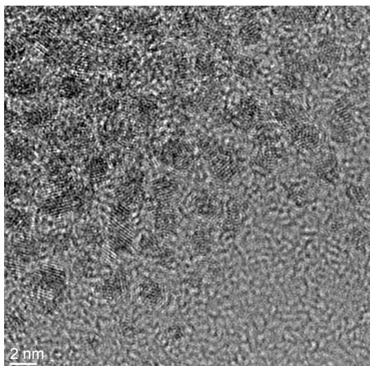
**Figure 8.** HRTEM image of **Pt1Ru4** nanoparticles.
