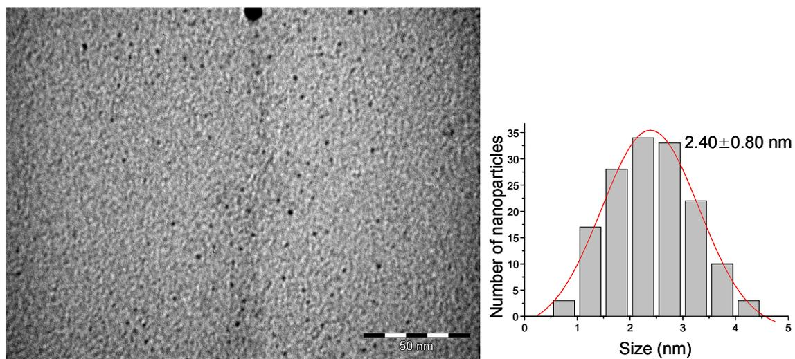
**Figure 11.** TEM image with the corresponding size histogram of **Ru1Pt2** nanoparticles after CAL hydrogenation.
