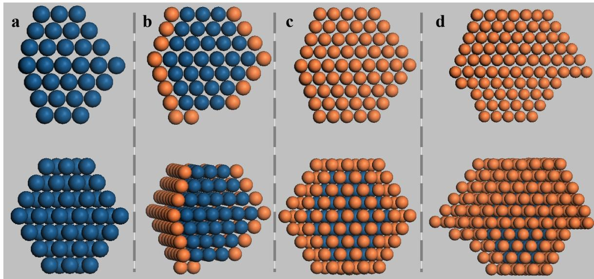
a) Nanoparticle model of monometallic Pt (111) nanoparticles (top along Y axis view and bottom with angles). Model containing 83 atoms (Empirical radius of platinum was used in the cluster model,  $1.35 \times 2 \times 6 = 1.62$  nm).
