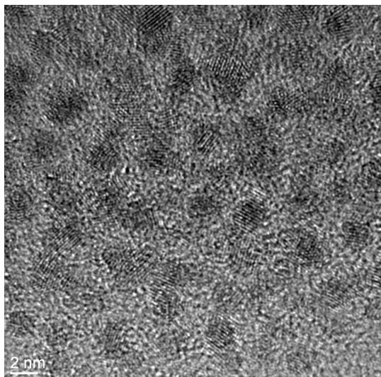
**Figure 7.** HRTEM image of **Pt1Ru2** nanoparticles.
