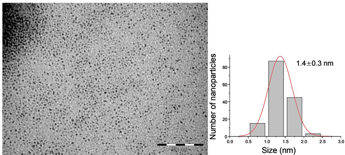
**Figure 14.** TEM image with the corresponding size histogram of **Pt1Ru1** nanoparticles after CAL hydrogenation.
