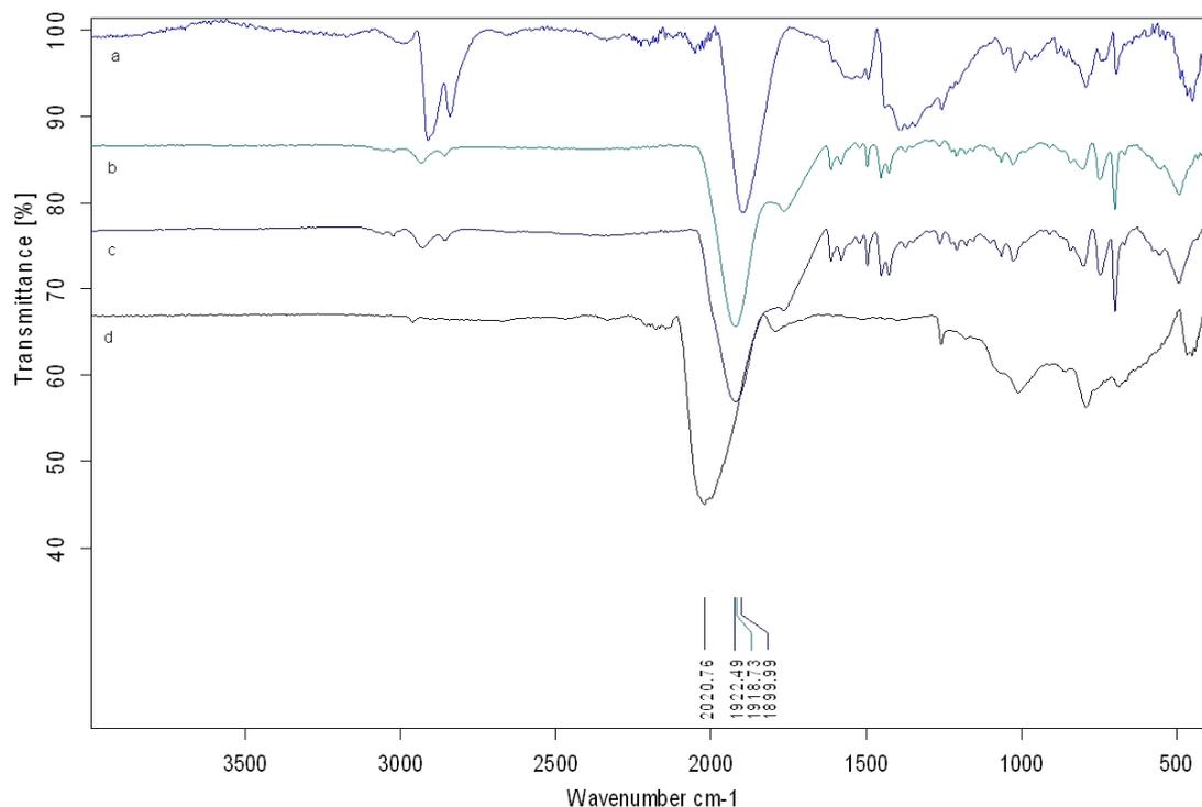
**Figure 9.** ATR-IR spectra for **PtRu** nanoparticles: a) **Pt1Ru4** (1899  $\text{cm}^{-1}$ ), b) **Pt1Ru2** (1918  $\text{cm}^{-1}$ ), c) **Pt1Ru1** (1922  $\text{cm}^{-1}$ ), and d) **Pt/CO** (2018  $\text{cm}^{-1}$ ).
