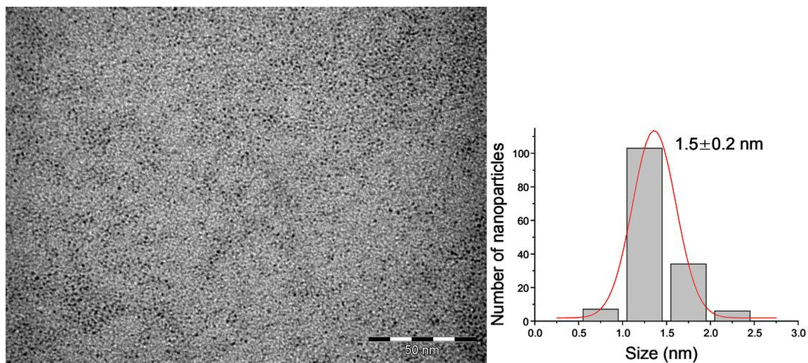
**Figure 15.** TEM image with the corresponding size histogram of **Pt1Ru2** nanoparticles after CAL hydrogenation.
