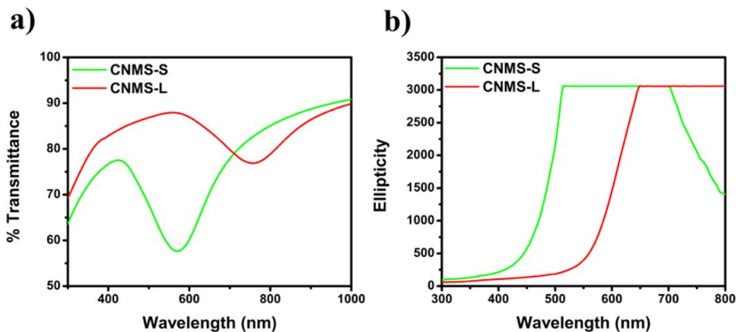
**Fig. S1.** (a) UV-Vis spectra of the CNMS-S and CNMS-L films showing the photonic band gap in both materials. (b) CD spectra of the CNMS-S and CNMS-L films. The spectra appear cut off since the peak are greater than the maximum detectable signal on the spectropolarimeter that was used.
