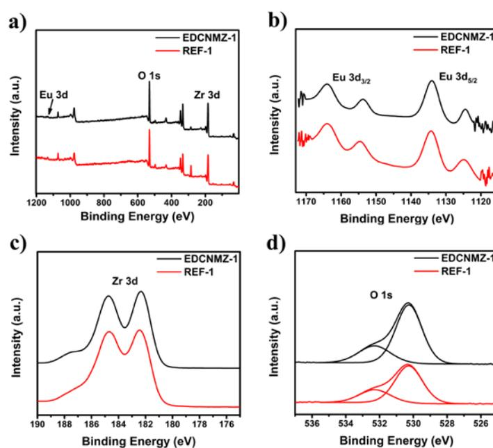
**Fig. S4.** (a) XPS survey spectra of EDCNMZ-1 and REF-1. (b) Deconvoluted XPS peaks of Eu3d. (c) Deconvoluted XPS peaks of Zr3d. (d) Deconvoluted XPS peaks of O1s.
