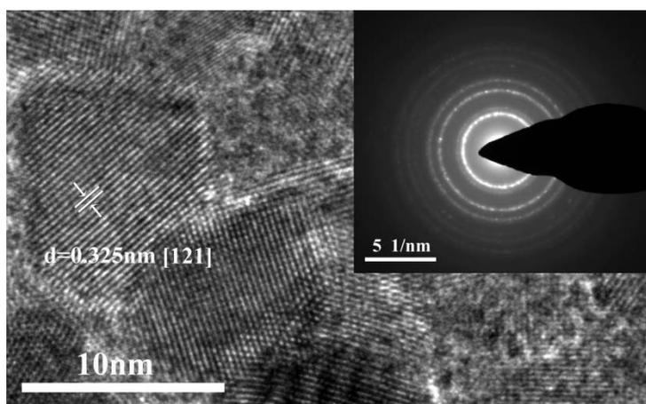
**Fig. S3.** HRTEM image of EDCNMZ-1 showing the presence of crystalline domains of  $\text{ZrO}_2$  with the average  $d_{121}$ -spacing of the lattice fringes around 0.325 nm; Inset is the SEAD of EDCNMZ-1.
