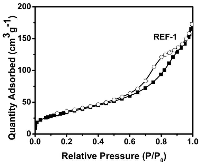
**Fig. S2.** Nitrogen adsorption-desorption isotherm of REF-1.
