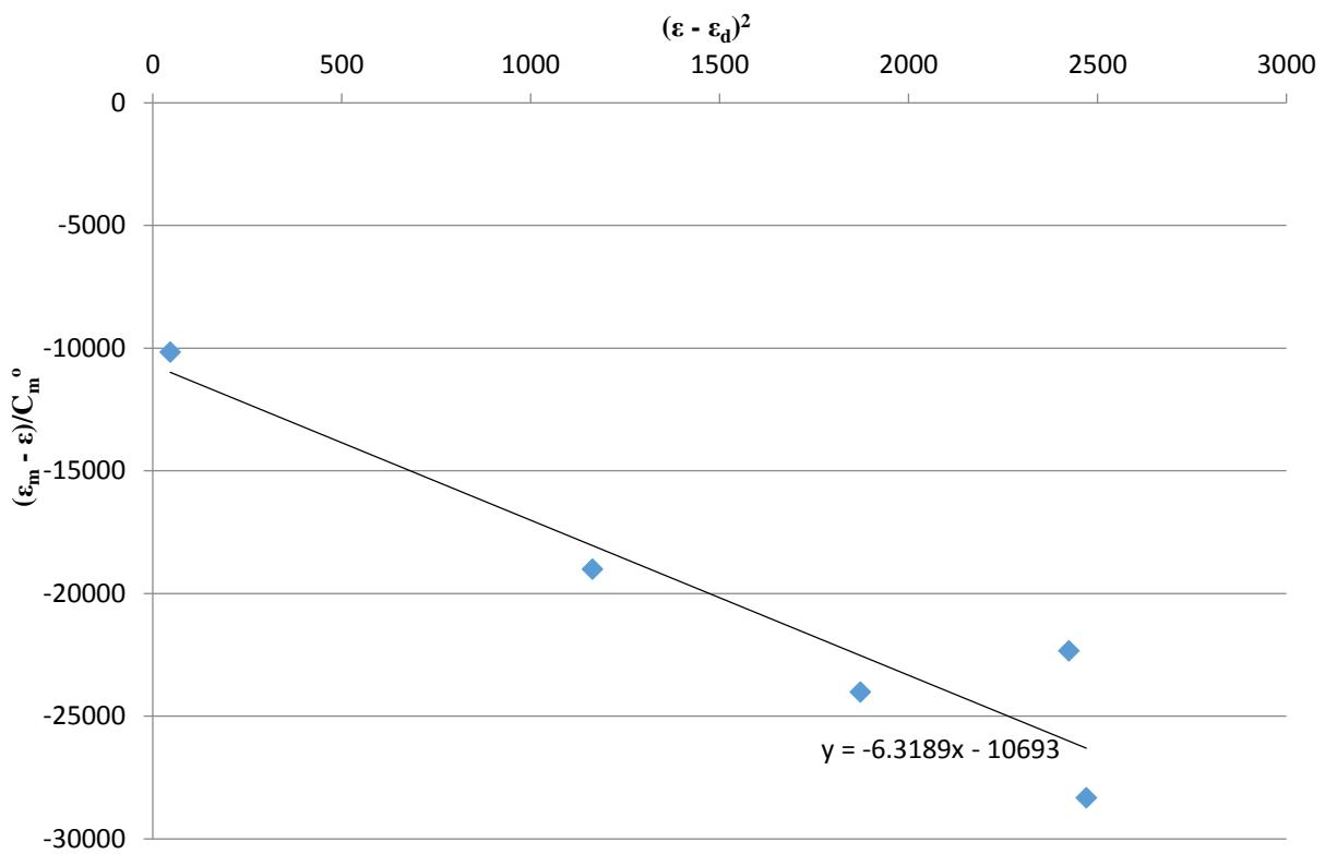
**Figure S9.** Linear fit to  $(\epsilon_m - \epsilon)/C_m^\circ$  vs.  $(\epsilon - \epsilon_d)^2$  at 632 nm for **2**.
