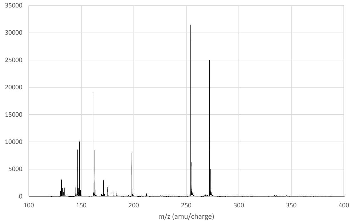
**Figure S2.** ESI-MS of BPYA in MeOH, the peak at 272 m/z corresponds to  $\text{LH}^+$ .
