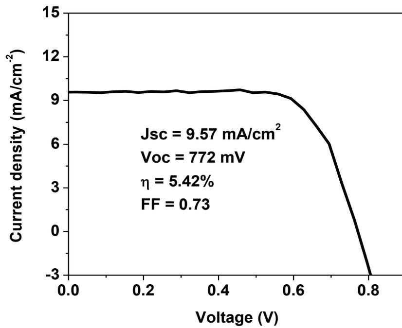
Figure S5: Current-voltage curve of dye sensitized solar cell with anatase TiO<sub>2</sub> nanoparticle (average size <25) film.
