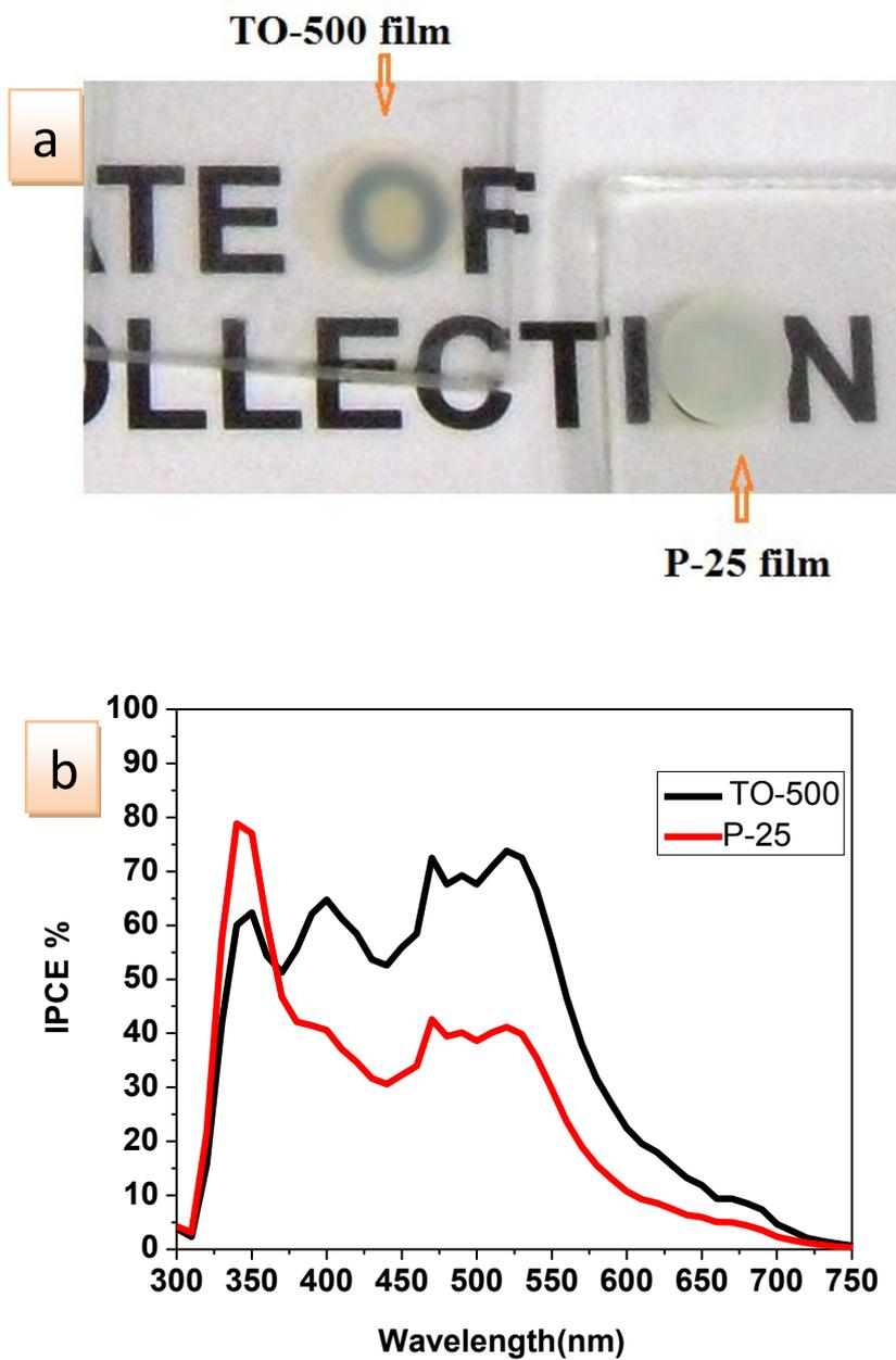
Figure S6: a) Photograph of TO-500 and P-25 films; b) IPCE of device A and B with TO-500 film and P-25 film respectively, which were fabricated and tested using similar experimental procedures.
