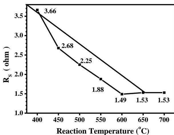
**Fig. S6** Equivalent series resistances extracted at 10 Hz (three-electrode system).
