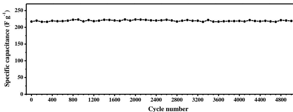
**Fig. S7** Cycling performance of TNNs-550 electrodes at a current density of 10 A/g (three-electrode system).
