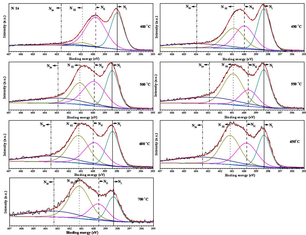
**Fig. S10** N1s XPS spectra of TNNs, showing four N configurations as deconvoluted (N<sub>i</sub>: pyridinic nitrogen, N<sub>ii</sub>: pyrrolic nitrogen, N<sub>iii</sub>: quaternary nitrogen, N<sub>iv</sub>: oxidized nitrogen).
