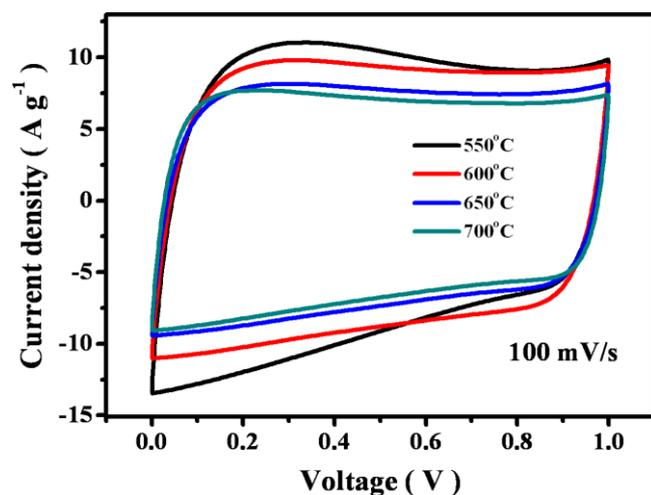
**Fig. S8** CV curves at the scan speed of 100 mV/s (two-electrode system).
