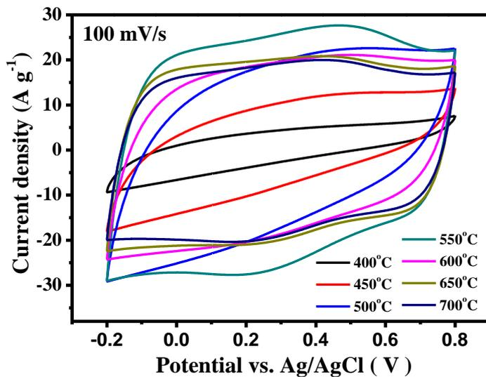
**Fig. S4** CV curves at the scan speed of 100 mV/s (three-electrode system).
