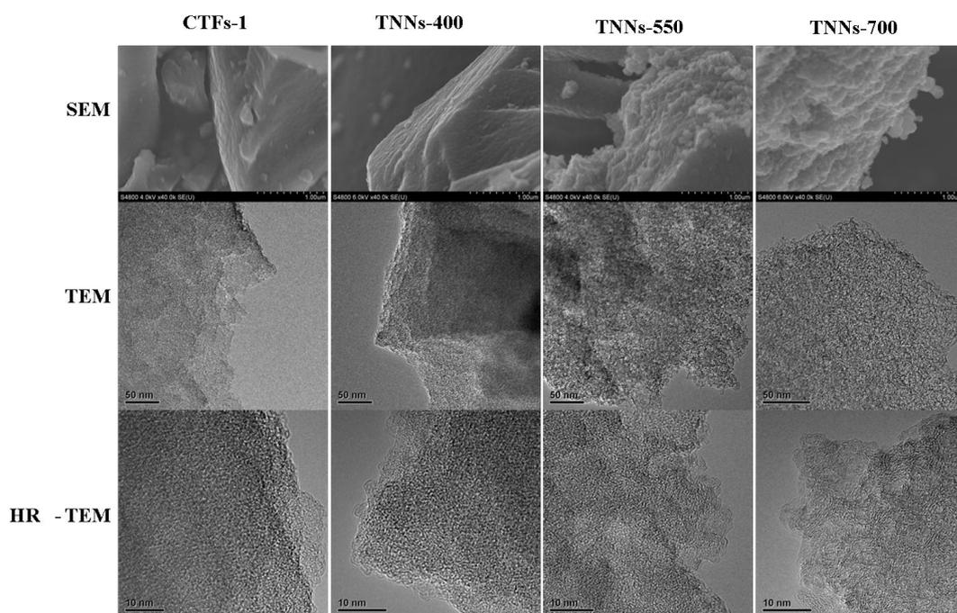
**Fig. S2** FE-SEM, FE-TEM, and high-resolution TEM images of CTFs-1, TNNs-400, TNNs-550, and TNNs-700.
