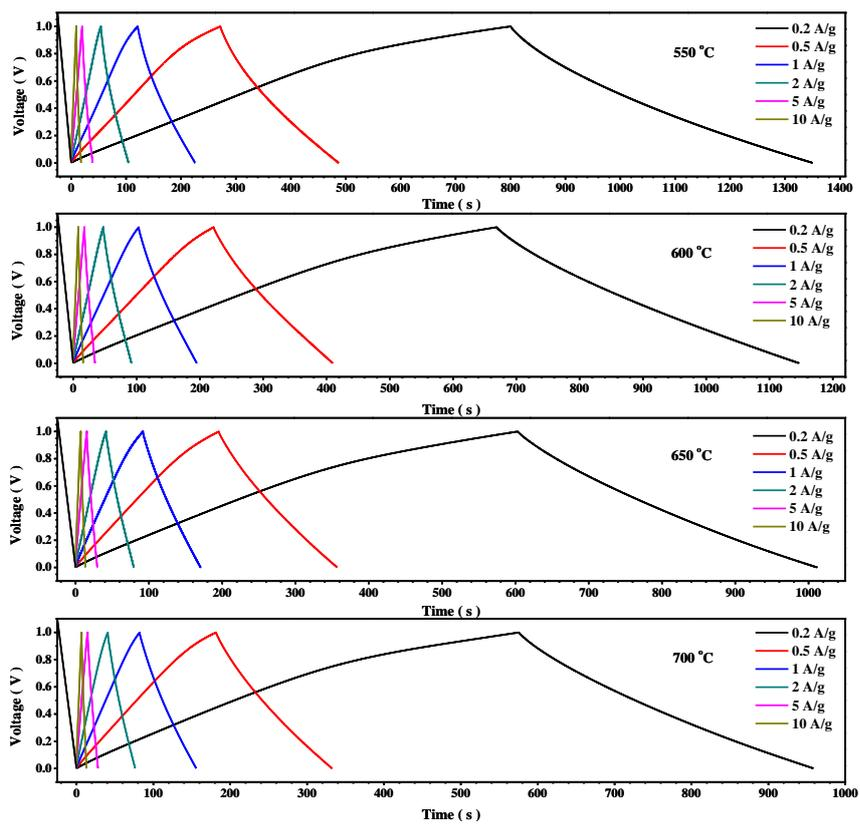
**Fig. S9** Galvanostatic charge-discharge curves at different current densities (two-electrode system).
