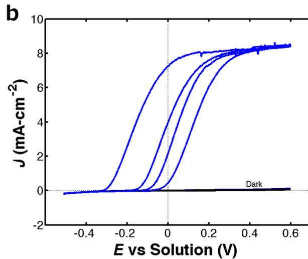
**Figure S 1:** Non-aqueous ferrocenium/ferrocene photoelectrochemical performance of a)  $\text{np}^+\text{-Si}$  and b)  $\text{n-Si}$  microwire arrays under  $100 \text{ mW cm}^{-2}$  of ELH-type W-halogen illumination.
