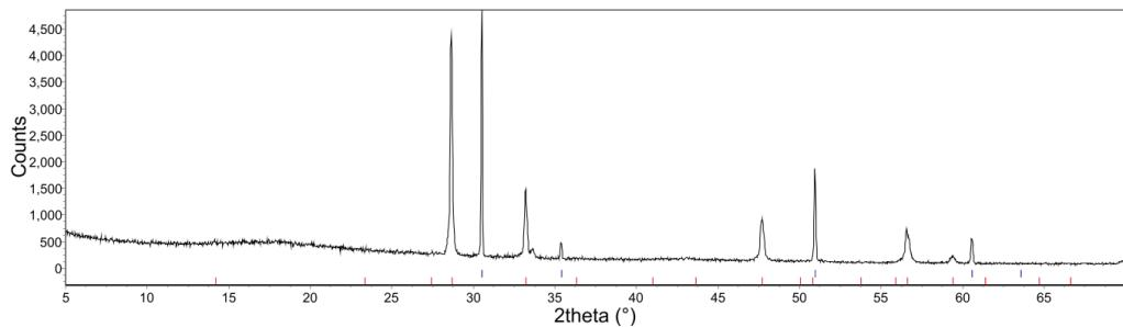
**Fig. S4** Powder X-ray diffraction pattern of  $\text{Li}_0\text{Mg}_{0.5}(\text{NH}_2)_6\text{Br} + 6\text{LiH}$  after TPD-MS experiment.
