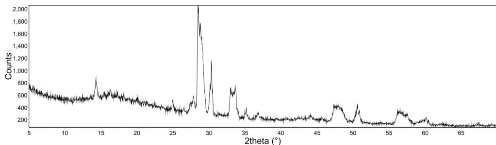
**Fig. S5** Powder X-ray diffraction pattern of  $\text{Li}_7(\text{NH}_2)_6\text{Br} + 6\text{LiH}$  after TPD–MS experiment.
