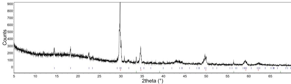
**Fig. S8** Powder X-ray diffraction pattern of  $3\text{Li}_2\text{NH} \cdot \frac{1}{2}\text{MgCl}_2$  after hydrogenation at  $300^\circ\text{C}$ , 100 bar  $\text{H}_2$ . Tick marks indicate peaks due to a rhombohedral  $\text{Li}_4(\text{NH}_2)_3\text{Cl}$ -like phase (blue),  $\text{LiCl}$  (red) and  $\text{Li}_2\text{O}$  (green).
