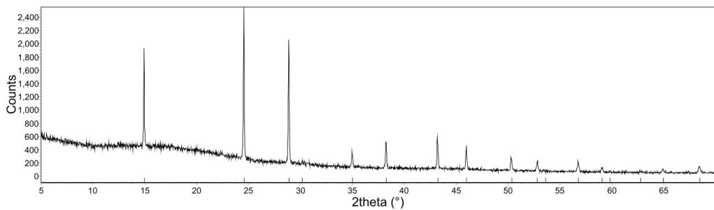
**Fig. S6** Powder X-ray diffraction pattern of  $3\text{LiNH}_2 \cdot \text{LiI} + 3\text{LiH}$  after TPD–MS experiment. Tick marks indicate peaks due to  $\text{Li}_5(\text{NH}_2)_2\text{I}$ .
