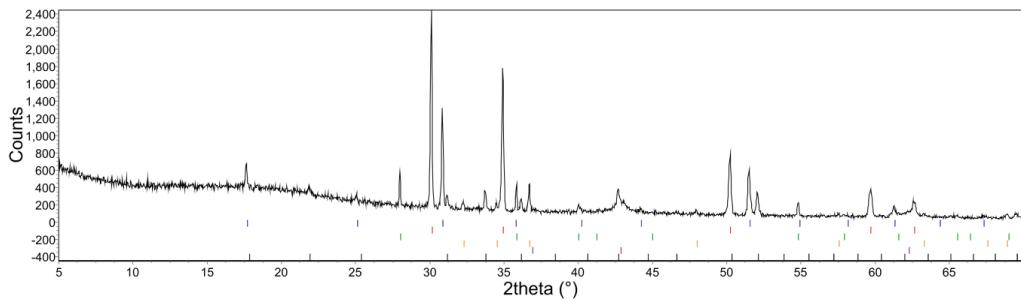
**Fig. S7** Powder X-ray diffraction pattern of  $2\text{Li}_3\text{Mg}_{0.5}(\text{NH}_2)_3\text{Cl} + 3\text{MgH}_2$  after TPD-MS experiment. Tick marks indicate peaks due to  $\beta\text{-Li}_2\text{Mg}(\text{NH}_2)_2$  (blue),  $\text{LiCl}$  (red),  $\text{MgH}_2$  (green),  $\text{Mg}$  (orange),  $\text{MgO}$  (purple) and  $\text{Mg}_3\text{N}_2$  (black).
