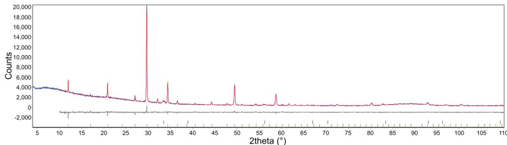
**Fig. S1** Preliminary Rietveld plot for  $\text{Li}_4(\text{NH}_2)_3\text{Cl}$ . Tick marks indicate peak positions due to  $\text{Li}_4(\text{NH}_2)_3\text{Cl}$  (green) and  $\text{Li}_2\text{O}$  (black).
