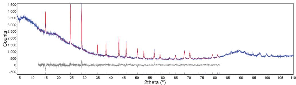
**Fig. S3** Preliminary Rietveld plot for  $\text{Li}_5(\text{NH})_2\text{I}$ . Tick marks indicate peak positions due to  $\text{Li}_5(\text{NH})_2\text{I}$ .
