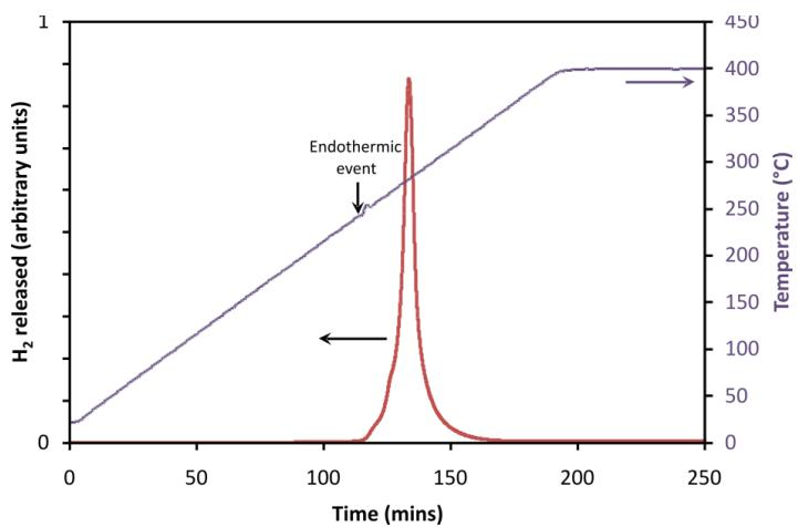
**Fig. S12** TPD–MS data for  $\text{Li}_6\text{Mg}_{0.5}(\text{NH}_2)_6\text{Br} + 3\text{MgH}_2$  showing an endothermic event in the temperature trace immediately prior to hydrogen release.
