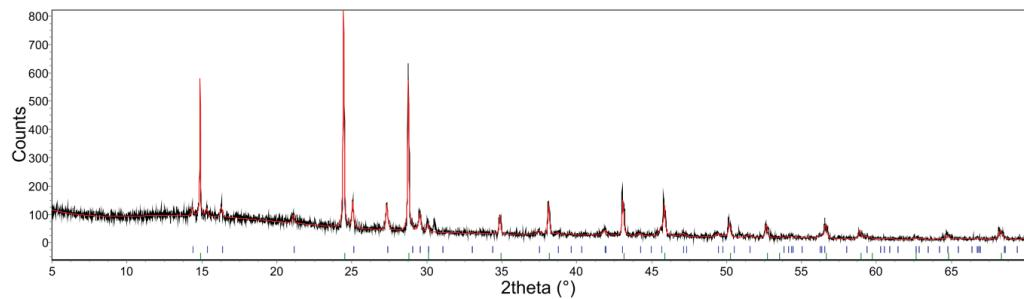
**Fig. S10** Observed (black) and calculated (red) powder X-ray diffraction pattern of  $3\text{Li}_2\text{NH}\cdot\text{LiI}$  after hydrogenation at  $200^\circ\text{C}$ , 100 bar  $\text{H}_2$ , for 1 hour. Tick marks indicate peaks due to  $\text{Li}_3(\text{NH}_2)_2\text{I}$  (blue, ~24.4 wt%) and  $\text{Li}_5(\text{NH}_2)_2\text{I}$  (green, ~75.6 wt%).
