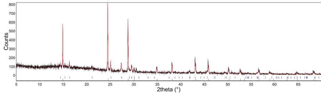
**Fig. S11** Observed (black) and calculated (red) powder X-ray diffraction pattern of  $3\text{Li}_2\text{NH}\cdot\frac{1}{2}\text{MgI}_2$  after hydrogenation at  $200^\circ\text{C}$ , 100 bar  $\text{H}_2$ , for 1 hour. Tick marks indicate peaks due to  $\text{Li}_2\text{Mg}_{0.5}(\text{NH}_2)_2\text{I}$  (blue, ~30.4 wt%) and  $\text{Li}_4\text{Mg}_{0.5}(\text{NH})_2\text{I}$  (green, ~69.6 wt%).
