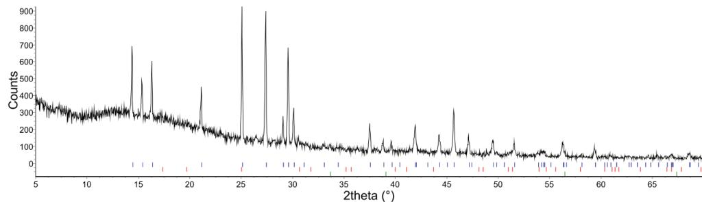
**Fig. S9** Powder X-ray diffraction pattern of  $3\text{Li}_2\text{NH}\cdot\text{LiI}$  after hydrogenation at  $300^\circ\text{C}$ , 100 bar  $\text{H}_2$ . Tick marks indicate peaks due to  $\text{Li}_3(\text{NH}_2)_2\text{I}$  (blue),  $\text{LiNH}_2$  (red) and  $\text{Li}_2\text{O}$  (green).
