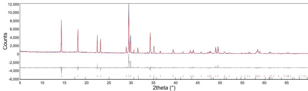
**Fig. S2** Preliminary Rietveld plot of N and Br positions in  $\text{Li}_7(\text{NH}_2)_6\text{Br}$ . Tick marks indicate peak positions due to  $\text{Li}_7(\text{NH}_2)_6\text{Br}$  (red) and  $\text{LiNH}_2$  (black).
