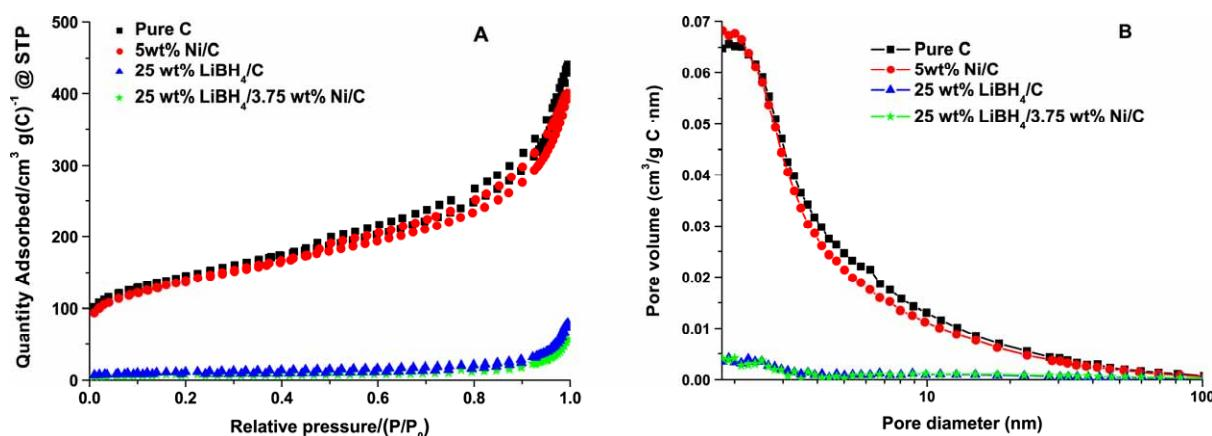
Figure S1. Nitrogen adsorption isotherms (A) and pore size distribution (B) of pure HSAG-500 carbon, 5wt% Ni/C, and nanocomposites 25LiBH<sub>4</sub>/C and 25LiBH<sub>4</sub>/3.75NiC.
