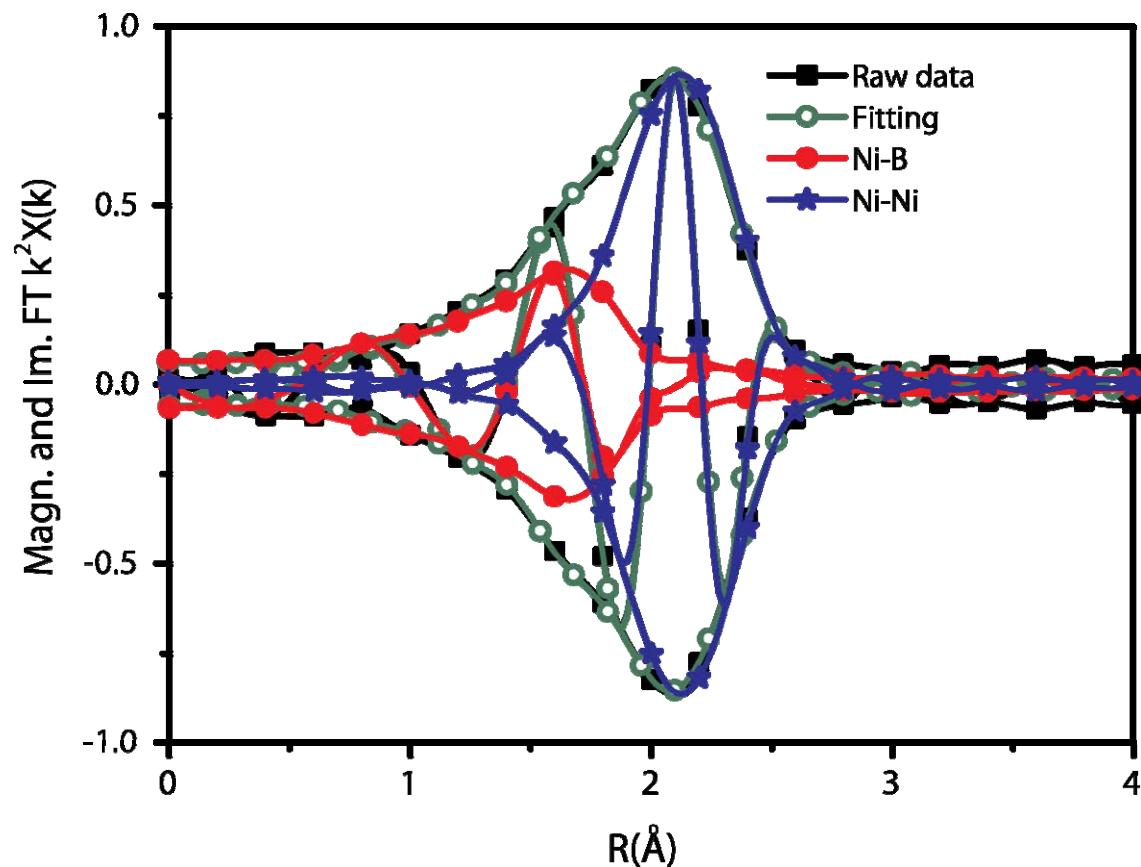
**Figure S4.** Magnitude and Imaginary part of the phase-uncorrected Fourier transformed  $\chi(k)$  for the as-synthesized LiBH<sub>4</sub>/Ni/C nanocomposites. The fit is optimized with  $\Delta k=3\text{--}13 \text{ \AA}^{-1}$  and  $\Delta R=1.2\text{--}3.0$  with the k-weighting parameter of 2. The individual contributions of Ni-B and Ni-Ni are also included.
