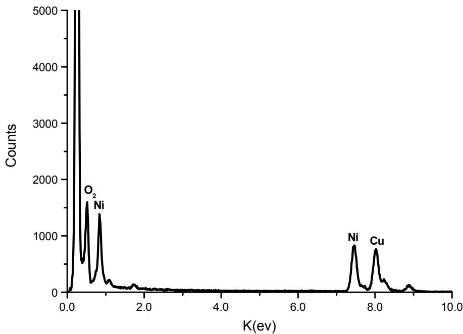
Figure S3 EDX signal from the LiBH<sub>4</sub>/Ni/C nanocomposites (sample 2B) showing the presence of Ni.
