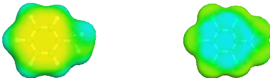
Fig. S2. Screening charge density maps of toluene (left) and perfluorotoluene (right), calculated by COSMOtherm.
