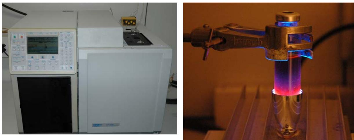
**Figure S30.** Left: gas chromatograph (Varian CP-3800) for recording chromatograms and monitoring  $\text{O}_2$  evolution during water oxidation; right: illumination of the reaction vessel by the light of a 470 nm high flux LED (Rhopoint Components LTD).
