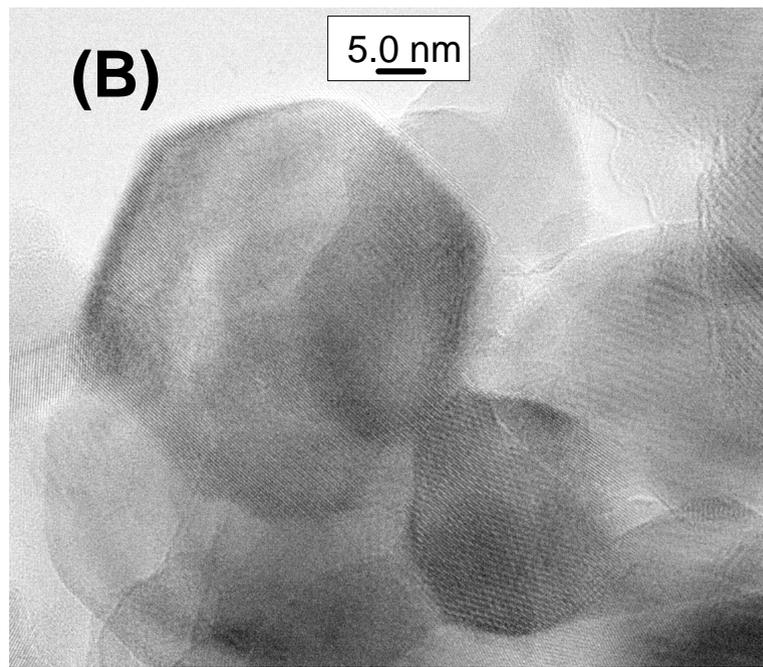
**ESI-Fig. 2** TEM images of mesoporous Al-Ti oxide calcined at 900 °C. Images (A) and (B) were taken at different locations in the sample.
