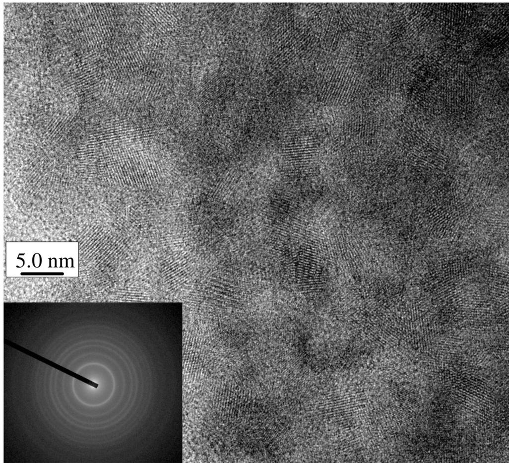
**ESI-Fig. 1** TEM image and electron diffraction pattern (inset) of mesoporous TiO<sub>2</sub> calcined at 400 °C.
