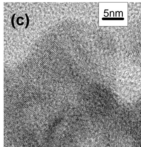
**ESI-Fig. 3** TEM images of mesoporous Ti-Nb oxide calcined at (a) 400 °C and (b, c) 530 °C.
