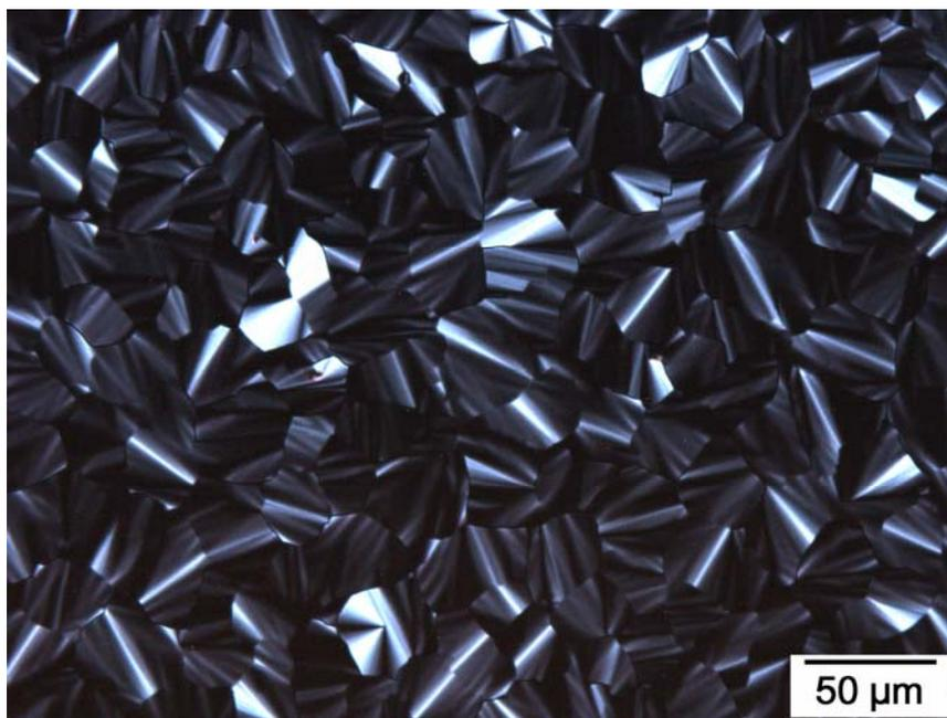
**Fig. S1.** (a) Optical texture of CoS12 at 80°C under cross polarizers, in its columnar hexagonal columnar LC phase, was measured upon cooling with the rate of 1°C/min.
