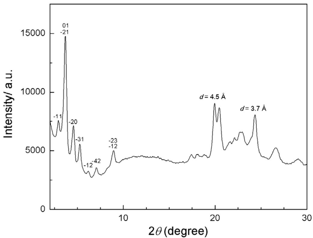
**Fig. S2.** 1D X-ray diffraction pattern of CoS12 measured at 25°C (solid phase).
