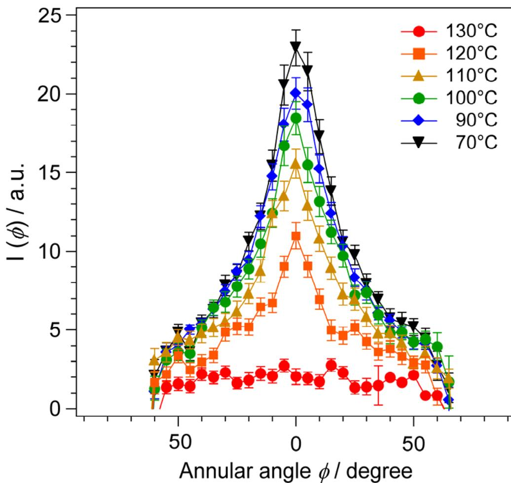
**Fig. S3.** Annular averaged SANS intensities of CoS12 measured at different temperature in the presence of an applied magnetic field of 1.0 T. The measurements were performed during cooling from the isotropic phase.
